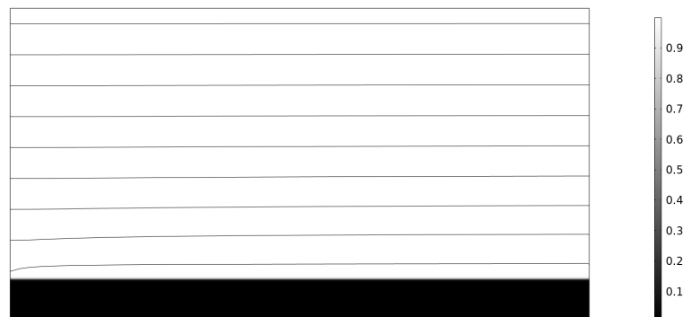
Figure B.3: Design geometry of the 2D-Plate-TF reference problem. Depicted is the projected pseudodensity field and streamlines of the velocity field for illustrative purposes.
