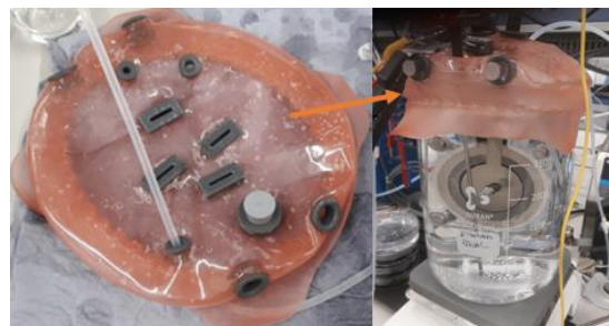
Figure 33: The hoody which will protect the researcher from airborne KCl particles and reduces the evaporation of water out of the electrolyte. The original silicone comes from IKEA®.
