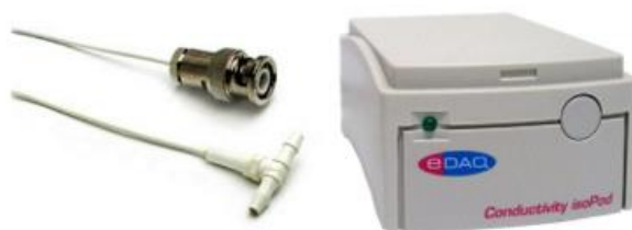
Figure 32: Picture of the eDAQ ET908 Flow-Thru Conductivity Electrode (left) for use of the EPU357 Conductivity isoPod™ with USB (right). Retrieved from the official website of eDAQ [119,120].
