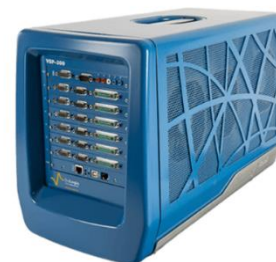
Figure 24: The EIS potentiostat Biologic VSP-300 [115].
