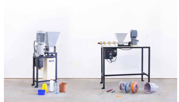
The open source plastic processing machines from Precious Plastic allow people from all over the world to make plastic products from their own waste.
