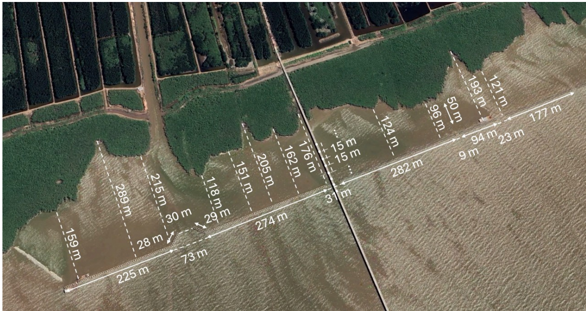
Figure 5.6: The spatial layout of the existing breakwater in the study area [23]
