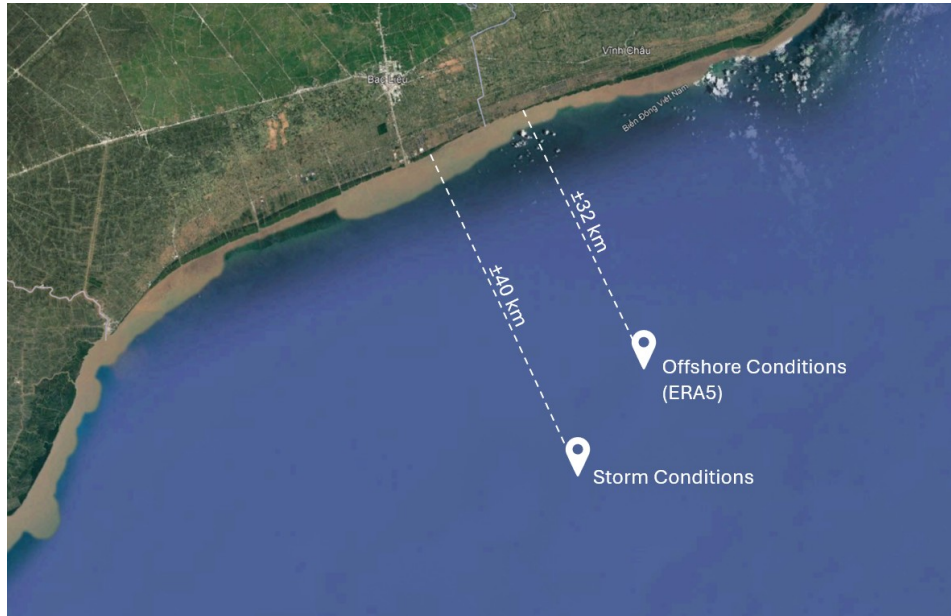
Figure B.4: Measurement locations for offshore hydrodynamic conditions and their distances from the shore [23]. One location represents the mean offshore conditions for summer and winter (approximately 32 km offshore at 9°N, 106°E), while the other marks the location for storm conditions (approximately 40 km offshore).
