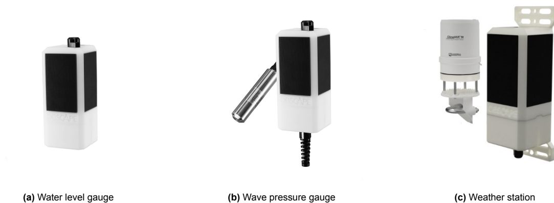
Figure A.1: Obscape monitoring instruments used for environmental data collection [60]. The water level gauge tracks tidal variations, the wave pressure gauge measures hydrodynamic forces, and the weather station records meteorological parameters such as wind speed, temperature, and atmospheric pressure.
