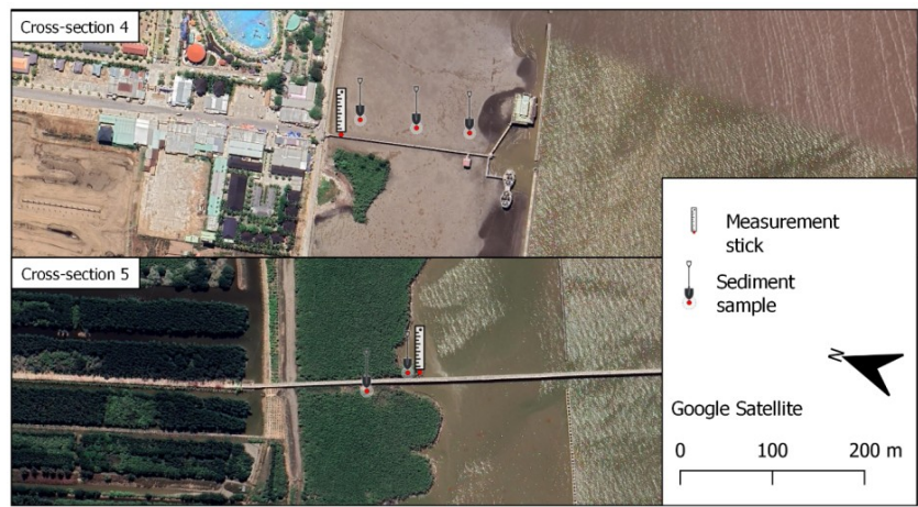
Figure B.10: Locations of the taken soil samples: Cross-section 4 in Nhà Mát and cross-section 5 at the Hòa Bình wind farm (study area) [6]
