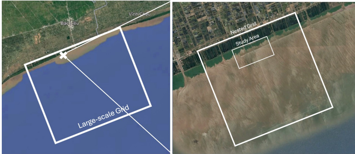
Figure 4.1: Large-scale and nested grid used in the Delft3D model [23].
