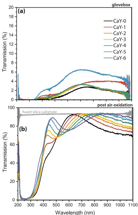
**Figure 1.** Optical transmission spectra for Ca-doped Y-based thin films (a) in the glovebox before oxidation and (b) post air exposure, showing the dihydride and oxyhydride phases, respectively. Samples CaY-0 to CaY-6 correspond to the Ca contents which vary from 0 to 36% (see Figure 2c).
