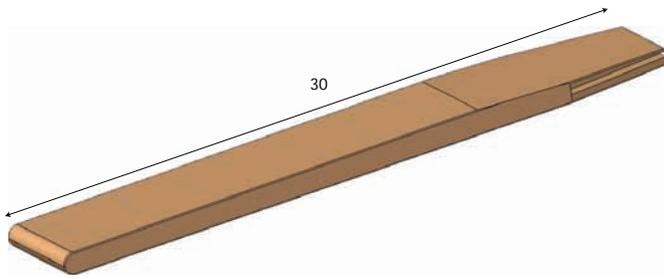
**Fig. 17:** Adhesive grasper: jaw. Two flat, rigid, rectangular jaws with rounded edges are chosen to prevent high surface pressures. The jaws are connected to the instrument by the cut in the back. The top of the jaw is sloping to allow actuation using a hollow tube
