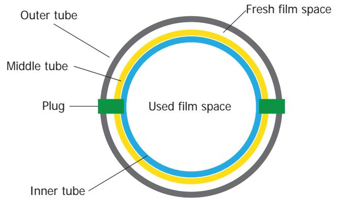
**Fig. 18:** Central shaft: cross section without middle tube (left) and with middle tube (right). Inner and outer tube are fixed using a plug. The middle tube slides across the inner tube to actuate the jaws. Fresh adhesive film is located between middle and outer tube, used adhesive film is located inside the inner tube
