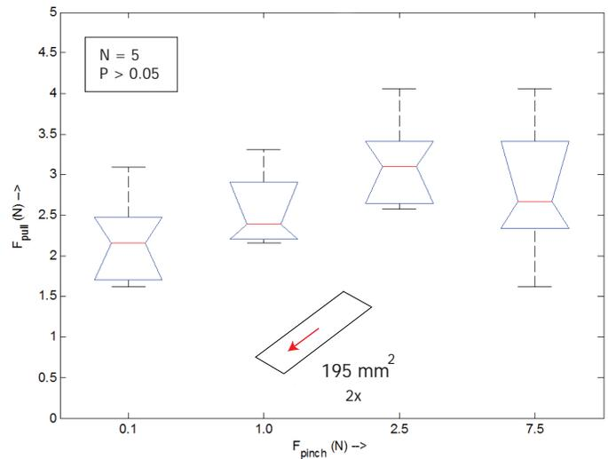
**Fig. 28:** Evaluation experiment: effect of pinch force on pull force for a contact area of  $390 \text{ mm}^2$  and applied pinch force of 0.1, 1.0, 2.5 and 7.5 N. The line in the middle of the box is the median, the upper and lower lines indicate the interquartile range, the whiskers extending indicate the spread
