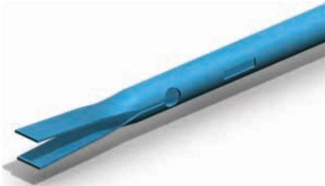
**Fig. 21:** Adhesive grasper: inner tube hinge. The end of the inner tube is sawed in, made flat and bend upwards, creating a material hinge and mounting point for the jaws. The round hole on the left is a relief cut for the material hinge. The square hole on the right is for the plug
