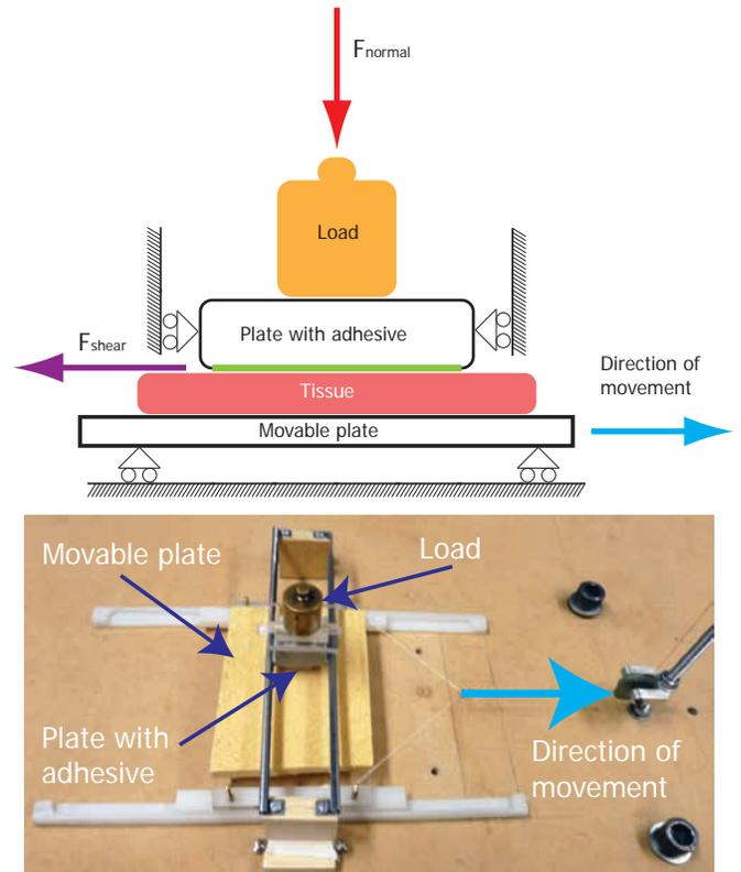
**Fig. 14:** Exploring experiment 2: set-up schematic (top), reality (bottom) to measure the maximum  $F_{shear,x}$  and  $F_{shear,y}$ . Adhesive film (100 mm<sup>2</sup> or 200 mm<sup>2</sup>) is fixed to a Plexiglas plate, which is placed on a piece of intestine. A load of 5, 15 or 30 kPa is placed on top of the plate with adhesive. Subsequently the movable plate is pulled to the right and the shear force is measured
