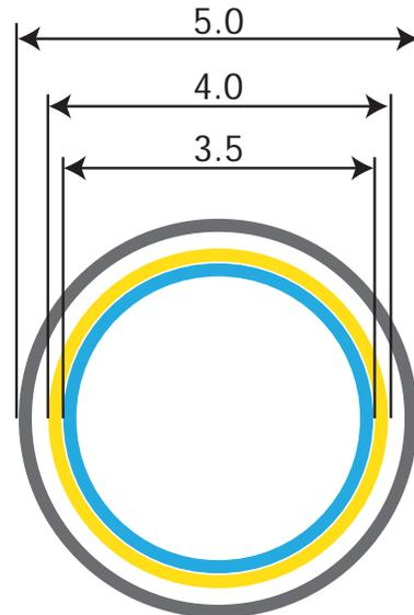
**Fig. 19:** Central shaft: cross section dimensions. For the outer tube (grey) a tube with 5mm outside diameter was used. For the outer tube (yellow) a tube with 4 mm outside diameter was used. For the inner tube (blue) a tube with 3.5 mm outside diameter was used. All tubes have a wall thickness of 0.25 mm. The distance between outer and middle tube is 0.25 mm
