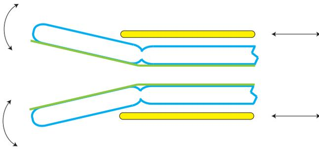
**Fig. 20:** Adhesive grasper: actuation schematic (left) and render (right). In the starting position the grasper is in open position. Pushing the middle tube (yellow) pushed forward across the inner tube (blue) forces the jaws to close
