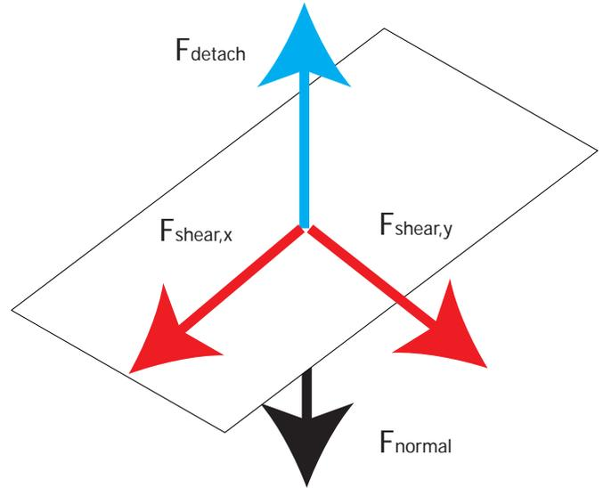
**Fig. 10:** Adhesive film: force directions. Adhesive film can generate detachment force and friction force, while for example a normal force can be applied to the film to enlarge the reel contact area
