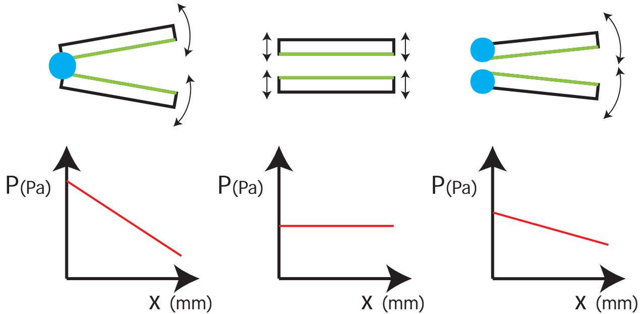
**Fig. 5:** Motion concepts and pressure on tissue (theoretical). Single hinge motion(left), parallel motion (middle) and combination motion (right)
