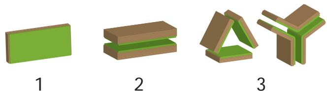
**Fig. 3:** Contact area: 1 jaw (left), 2 jaws (middle) and 3 jaws (right). Adhesive film is shown in green.
