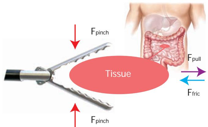
**Fig. 1:** Forces on tissue: during safe grasping friction force ( $F_{fric}$ ) = pull force ( $F_{pull}$ ) and the generated friction force ( $F_{fric}$ )  $\leq$  maximum friction force ( $F_{fric,max}$ )
