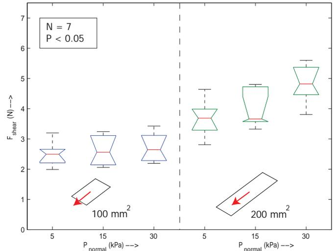
**Fig. 16:** Exploring experiment 2: effect of size of contact area, for a contact area of 100 mm<sup>2</sup> and 200 mm<sup>2</sup> and  $P_{\text{normal}}$  of 5, 15 or 30 kPa. The line in the middle of the box is the median, the upper and lower lines indicate the interquartile range, the whiskers extending indicate the spread
