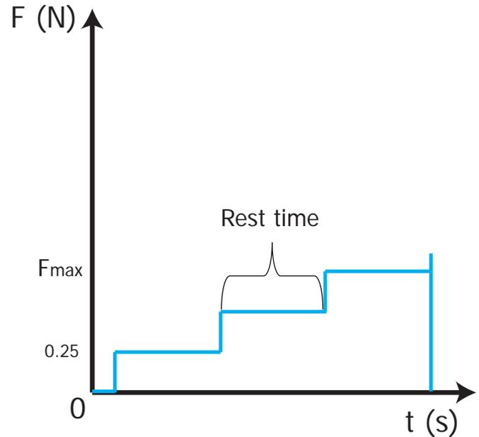
**Fig. 11:** Exploring experiment 1: force profile. Detachment force was increased in steps of 0.25 N using a rest time of 15 or 60 seconds to have a reasonable estimate of the maximum detachment force, within an acceptable experiment time. A minimum rest time of 15 seconds was required to observe if peeling occurred. A maximum rest time of 60 seconds was used, as stated in Section I C
