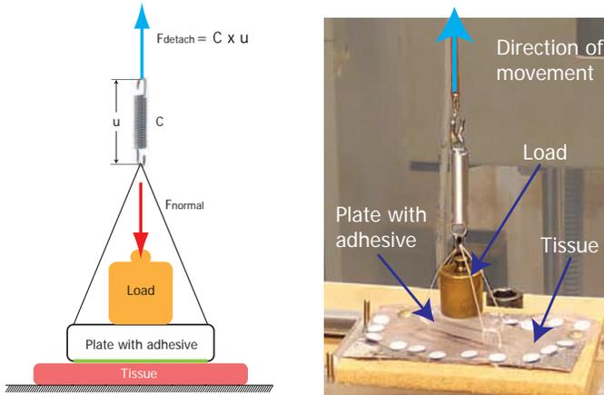
**Fig. 12:** Exploring experiment 1: set-up schematic (left), reality (right) to measure the maximum detachment force. Adhesive film ( $200 \text{ mm}^2$ ) is fixed to a Plexiglas plate, which is placed on a piece of intestine. A load of 5 kPa is placed on top of the Plexiglas plate. Next a stepwise increasing detachment force is applied and measured
