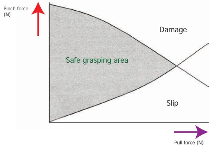
**Fig. 2:** A model of the combination of pinch force and pull force leading to slip, damage, or safe grasping of tissue. For safe tissue manipulation the pinch force needs to be high enough to prevent tissue slip, which is indicated by the lower boundary of the safe grasping area. Pull force introduces tension in the tissue, which lowers the maximum allowable pressure on the tissue. Any combination of pull and pinch force above the upper boundary of the safe grasping area will cause damage [10]
