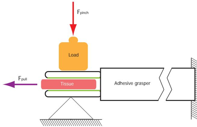
**Fig. 27:** Evaluation experiment: set-up (schematic) to measure the maximum pull force. The prototype of the adhesive grasper is loaded with adhesive film (resulting in a contact area of  $390 \text{ mm}^2$ ). Subsequently a pinch force of 0.1, 1, 2.5 or 7.5 N is applied and the tissue is pulled to the left, while the pull force is measured
