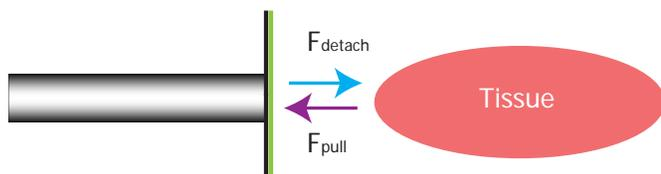
**Fig. 9:** Concept of adhesive grasper using a single contact surface (schematic). Adhesive film has to generate detachment force
