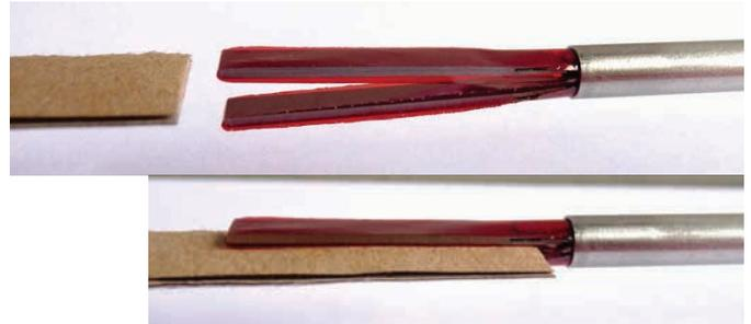
**Fig. 26:** Adhesive grasper: grasping. Tissue is positioned between the jaws of the grasper and the jaws are closed. The tissue is released by opening the jaws after which the tissue will release. After release of the tissue, the adhesive film is refreshed
