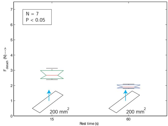
**Fig. 13:** Exploring experiment 1: effect of rest time on detachment force, for contact area of  $200 \text{ mm}^2$  and  $P_{normal}$  5 kPa. The line in the middle of the box is the median, the upper and lower lines indicate the interquartile range, the whiskers extending indicate the spread
