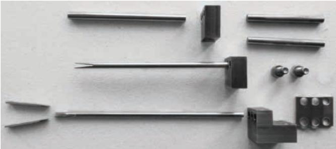
**Fig. 25:** Adhesive grasper: exploded view
