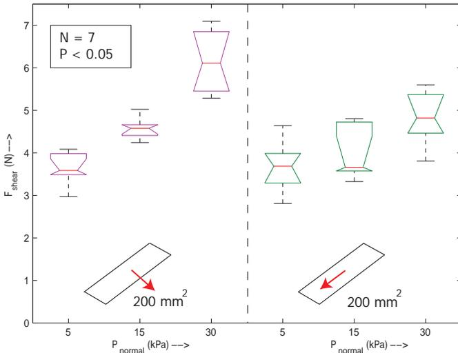
**Fig. 15:** Exploring experiment 2: effect of direction of displacement, for a contact area of 200 mm<sup>2</sup> and  $P_{\text{normal}}$  of 5, 15 or 30 kPa. The line in the middle of the box is the median, the upper and lower lines indicate the interquartile range, the whiskers extending indicate the spread
