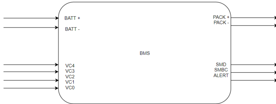
Figure 3.2: Top level overview of the BMS
