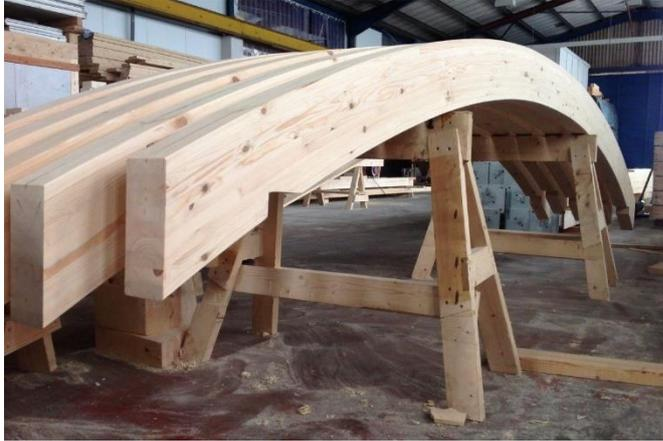
Figure 11 - Curved glued laminated beams [16].
