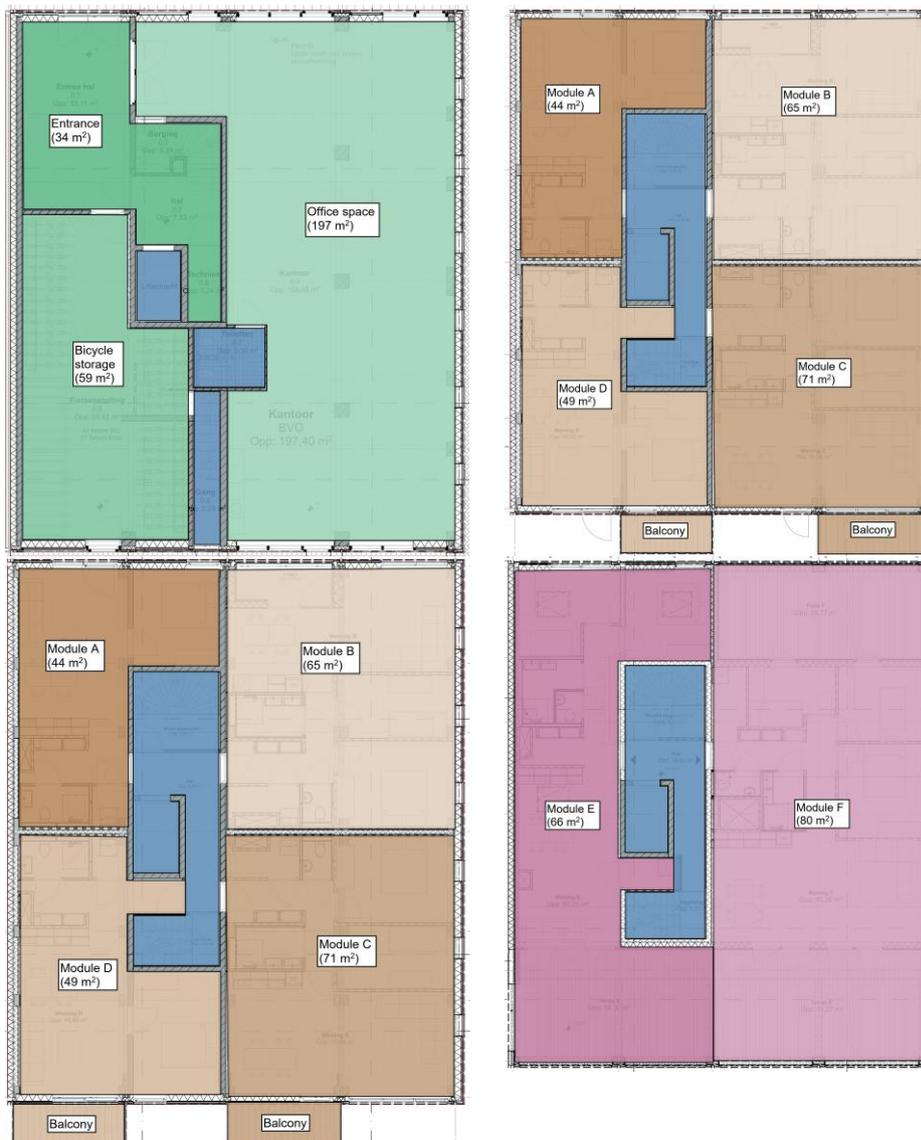
Figure 47 – Functional layout of the ground floor (top left), floors 1,3&5 (top right), floors 2&4 (bottom left) and floor 6 (bottom right).
