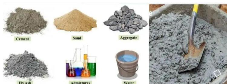
Figure 35 - Composition of raw materials concrete [44].
