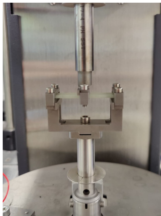
(b) DCB tooling on the TA Instruments RSA-G2.
