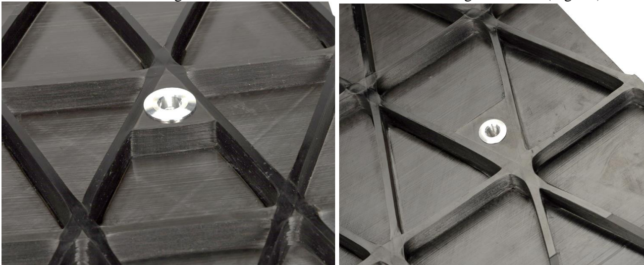
Fig. 11. Attachment zones with bonded inserts implemented into the demonstrator structure: Left – through bolt with a larger insert. Right – smaller insert for a blind hole.
