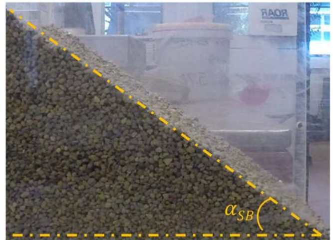
Fig. 4. Shear angle in the shear box test.
