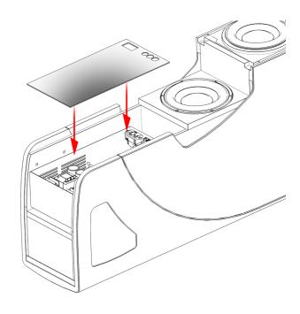
12. Electronics housing is closed using bolts.
