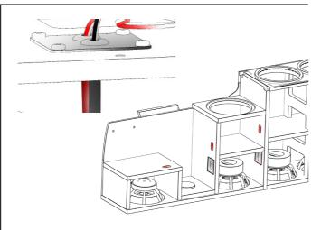
8. Metal speaker connection plates are fastened for the rear-sub, low-mid, and mid-driver.
