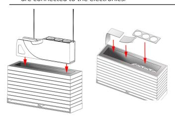
15. If the speaker passes all test, it is packed for trasnportation and the back panels are mounted.
