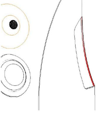
FIGURE 54. ALUMINUM EDGE STICKING OUT
