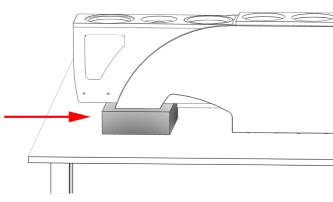
1. The cabinet is laid on its backside on a workbench; the rear top part is supported by custom-made wooden support.
