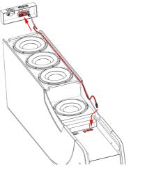
13. The connectors at the bottom of the speaker are connected to the electronics.
