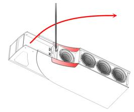
14. The speaker is tilted using the top pulley connection and the side roasters are mounted. The speaker is ready for performance tests.
