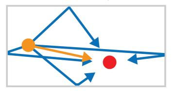
FIGURE 11. A SOURCE (ORANGE), LISTENER (RED), DIRECT (ORANGE) AND INDIRECT SOUND (BLUE) (K.AJ. KNAAPEN, 2014)
