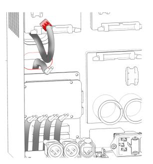
11. Speaker cables are led through the electronics housing and connected to the amplifiers.
