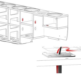
2. Cable plates for the front sub and low-mid compartment are screwed into the cabinet. The cable for the mid-driver is put through the plate not yet fastened.
