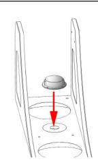
5. The tweeter is connected to the front baffle by four bolts.
