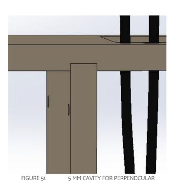
LOCATED TO ATTACH FRONT BAFFLE TO CABINET
