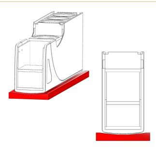
6. The front baffle is then placed flat on a second workbench. Positioned upon another support structure to divide the forces on the curved front baffle. The cabinet is then rotated and placed upon the front baffle. The ten bolts are then fastened to secure the front baffle to the cabinet.
