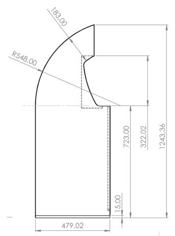
FIGURE 58. DIMENSIONS OF THE SOLID OAK LEFT SIDE PANEL
