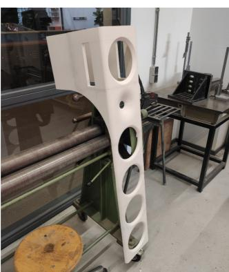
FIGURE 43. FIRST VERION OF 3D PRINTED FRONT BAFFLE
