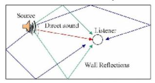
Figure 2: When listening to conventional speakers, you listen to the direct sound together with all in-room reflections
