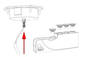
9. Rear speaker drivers and tweeter are connected to the cable and bolted into the cabinet.
