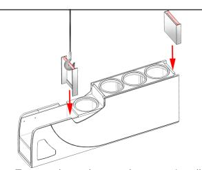
7. Two steel attachment plates are installed to accommodate lifting the body with a roof-mounted pulley.
