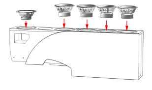
3. All front speaker drivers -except the tweeter- are connected and bolted onto the cabinet.
