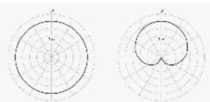
Figure 1: Omnidirectional radiation (left) versus Cardioid radiation (right) pattern of sound
