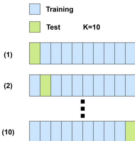
Figure 4.2: Schematic overview of the 10-fold cross-validation method. The test-set fraction (10 %) is shown in green and the training-set fraction (90 %) in blue. The process is repeated 10 times by iteratively selecting a new combination of training and test catchments.
