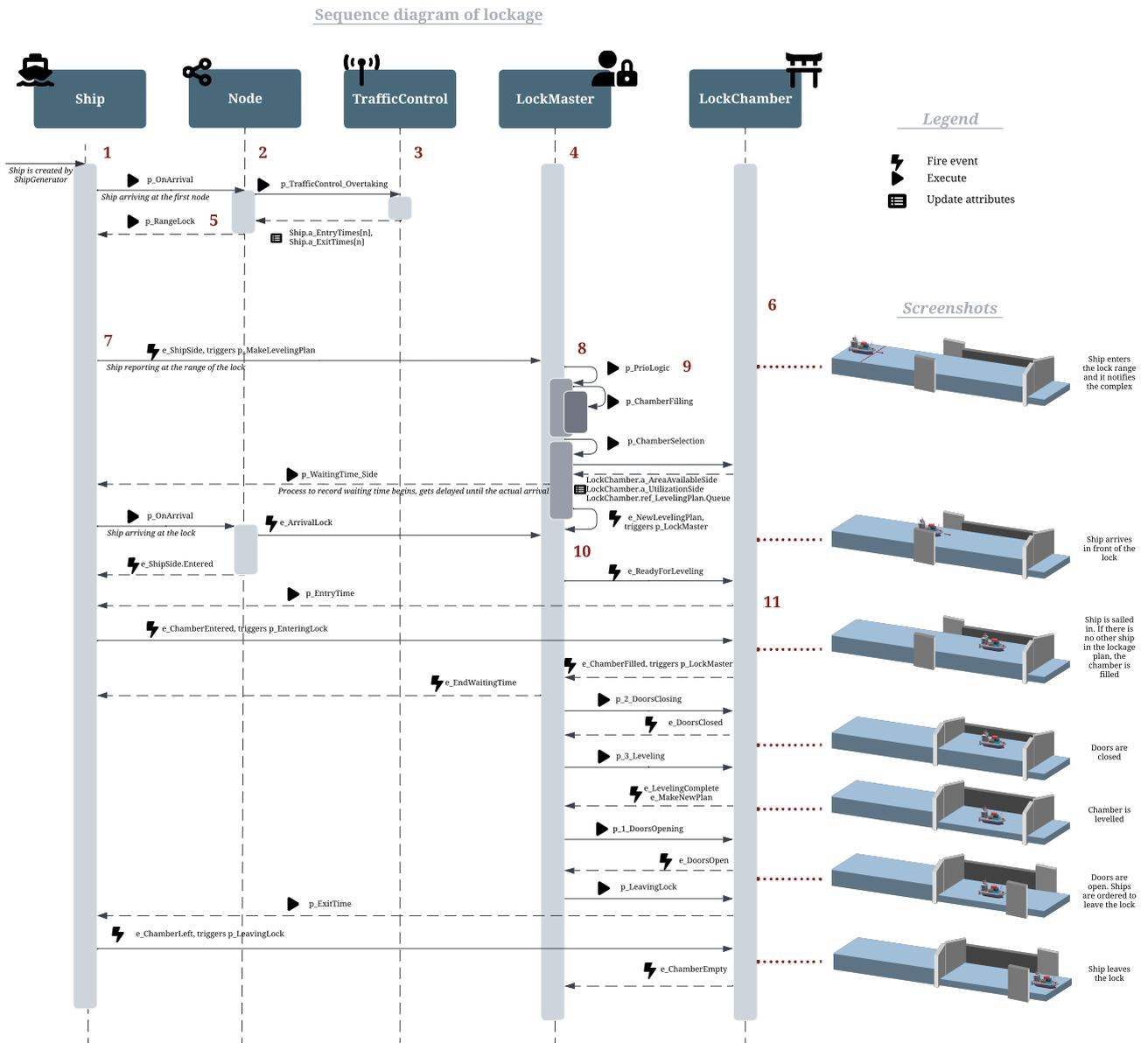
Figure F.2.: Sequence diagram of lockage
