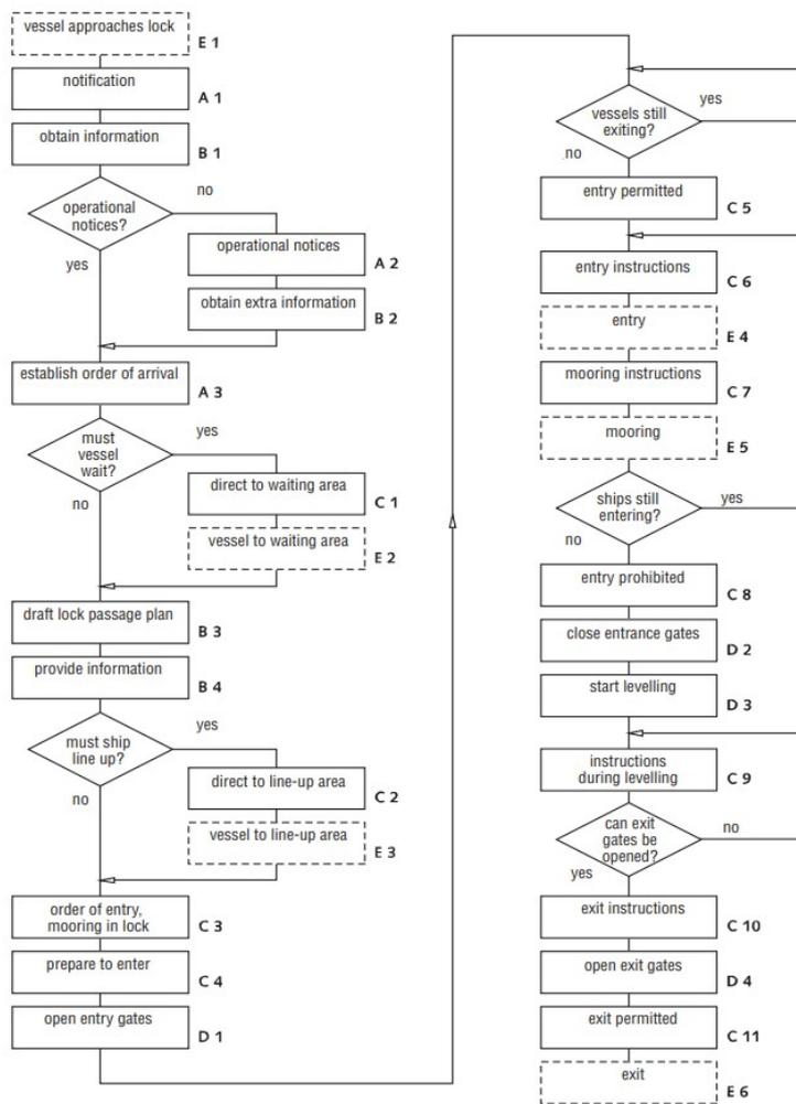
Figure C.1.: Flow diagram of lock passage of a vessel
