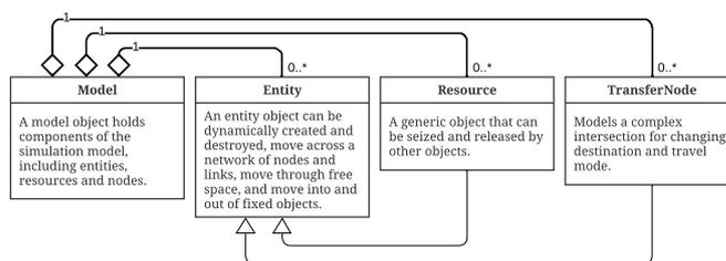
Figure F.1.: UML Class Diagram
