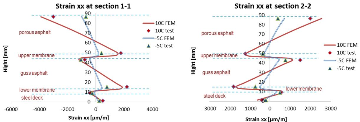
**FIGURE 16 Transversal strain at section 1-1& 2-2 (10 °C and -5 °C)**
