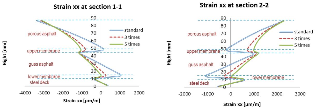
**FIGURE 14 Transversal strain at section 1-1 & 2-2 (membrane stiffness varies)**
