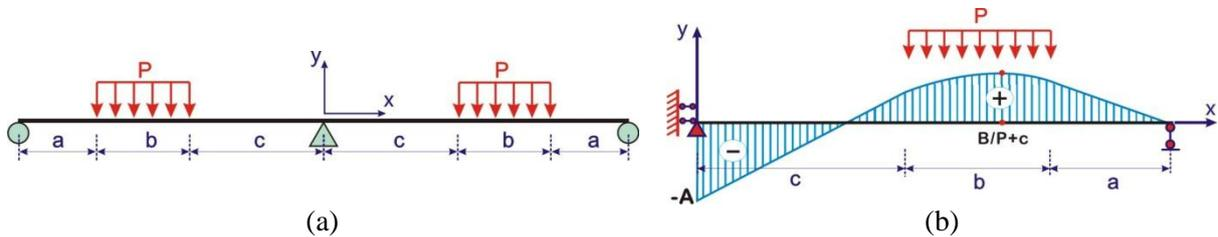
52 **FIGURE 2 (a) Beam model of 5PBT for analytical study; (b) Half of the model due to symmetry**
