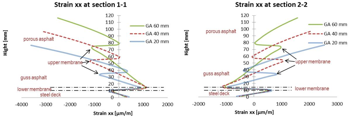
**FIGURE 11 Longitudinal strain at section 1-1 & 2-2 (GA thickness varies)**
