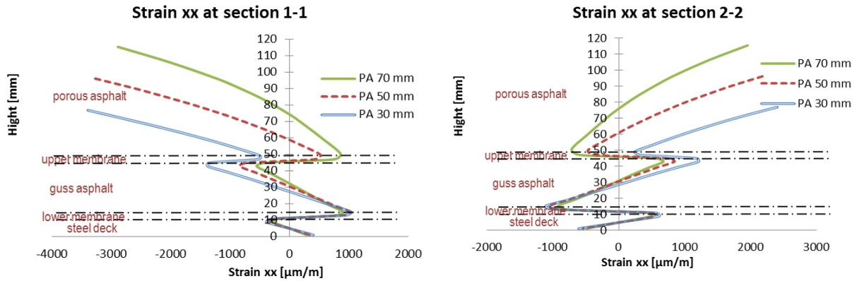
**FIGURE 9 Transversal strain at section 1-1 & 2-2 (PA thickness varies)**
