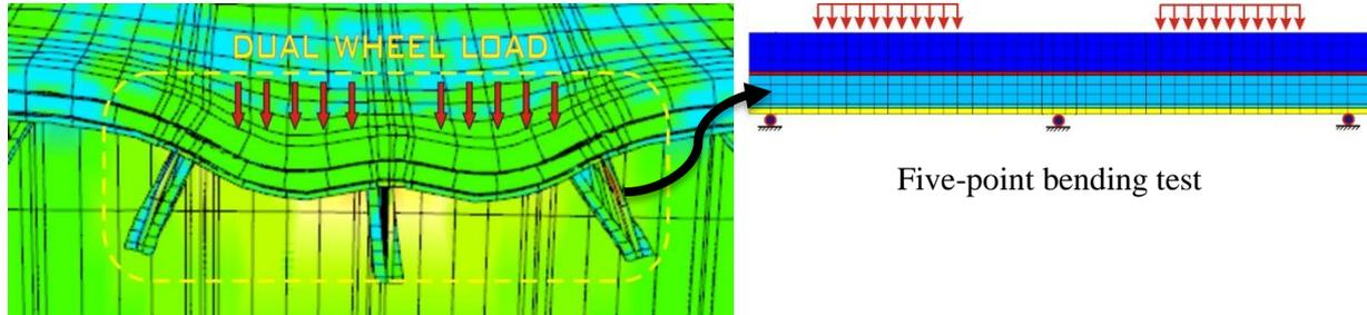
43 **FIGURE 1 Schematic show of a dual wheel load on OSDB and 5PBT**
