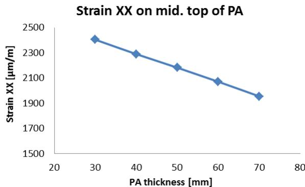
**FIGURE 10 Maximum transversal tensile strain on top of PA (PA thickness varies)**
