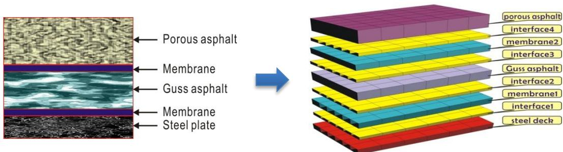
80 **FIGURE 4 Schematic diagram of the FE surfacing layers**
