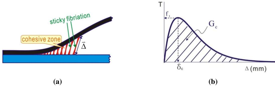
**FIGURE 7(a) Schematic of traction separation at contact interface; (b) Schematic traction-separation relation**
