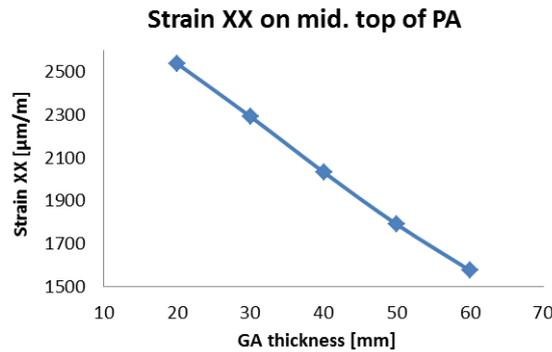
**FIGURE 12 Maximum tensile strain on top of PA (GA thickness varies)**
