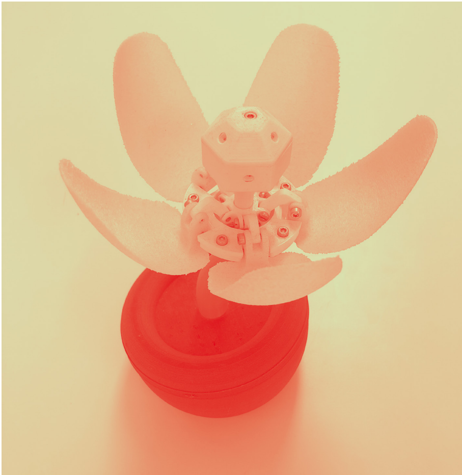
Fig. 40: Blooming Flower Night Night light designed by J. Suter (2023) to be easily 3D printed with minimal material and component costs.
