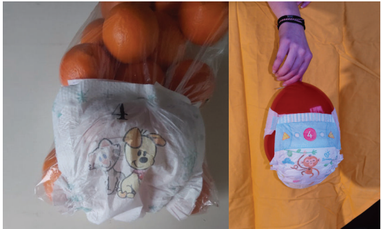
Figure 67) The test was performed with both a bag of oranges (to test movement) as well as inflating a balloon little by little (to test stretch)
