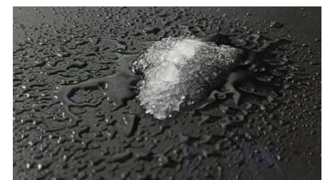
Figure 31) Fossil-based SAP absorbing water.
