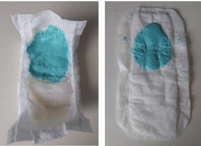
Figure 73) The results of the inlay test. Top left inlay with elastic, no leaks. Top right inlay with wings, no leaks. Bottom left, inlay without wings or elastics, leakage.
