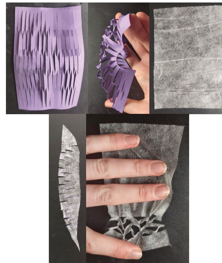
Figure 38) Tests done with paper and non-woven to create elastic material.
