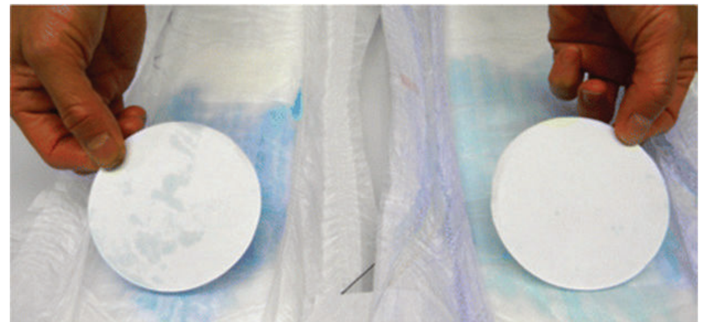
Figure 07) Rewetting comparison. (Helmes et al., 2014) As most diapers differ in composition, they also have different retention qualities. In the image can be seen that the retention of the diaper on the left is much lower than the diaper on the right. The rewetting value is therefore higher on the left, which will increase the risk of diaper dermatitis.
