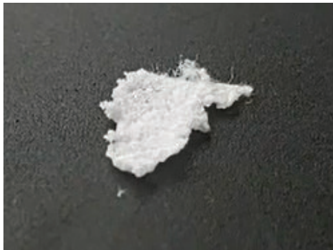
Figure 33) SAP granulate held together with adhesive.
