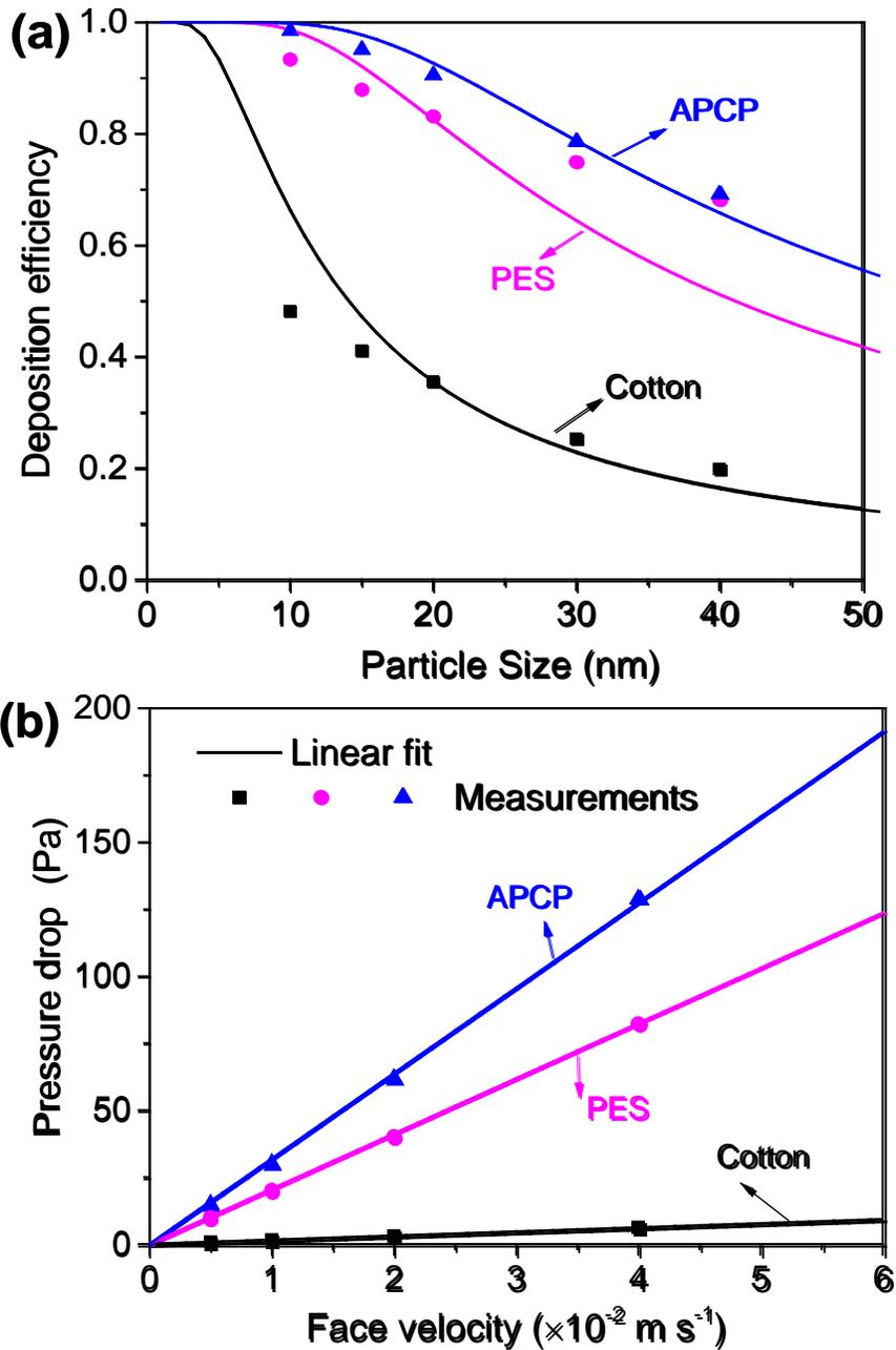
**Figure 3.** Variation in filtration performance of the textiles. (a) deposition efficiency as a function of particle diameter for a face velocity of  $0.02 \text{ m s}^{-1}$ . The curves represent predictions using equation (1), whereas the symbols correspond to the deposition measurements. (b) flow pressure drop across the textiles as a function of face velocity.
