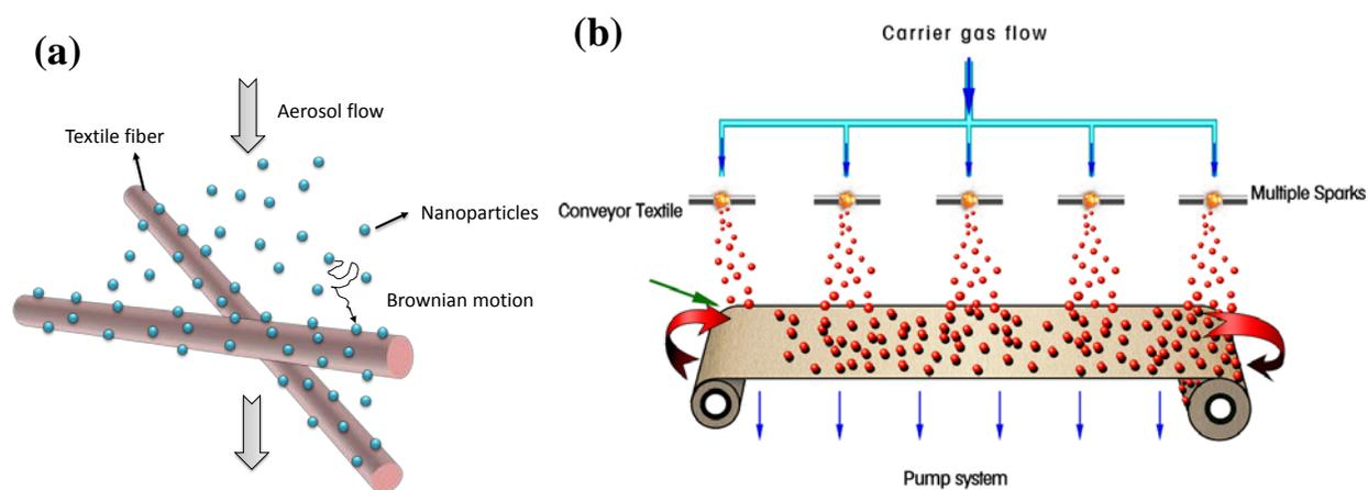
**Figure 1.** Illustration of the fabrication process. (a) An aerosol flow is passed through the textile, where the NPs collide and stick to the fibers by van der Waals forces. The NP-fiber collision is caused by the NP Brownian motion. (b) Conceptual design of a simple, scalable and green route for textile nanofinishing achieved by integrating electrical discharges for the synthesis of NPs into roll-to-roll textile production.
