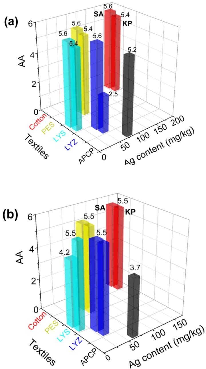
**Figure 7.** Antibacterial activity (AA) of the textiles treated with Ag NPs against *Staphylococcus Aureus* (SA), and *Klebsiella Pneumoniae* (KP), as shown respectively in the left and right rectangular columns of the same textile. (a) antibacterial activity of non-washed textiles versus Ag content; (b) antibacterial activity of washed textiles (three cycles, only five cycles for APCP) versus Ag content.
