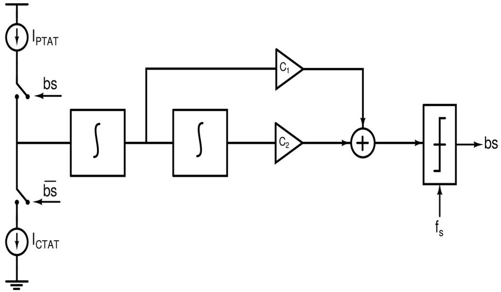
Figure 4.1: Diagram of the linear charge-balancing feed-forward 2<sup>nd</sup> order  $\Delta\Sigma$  modulator
