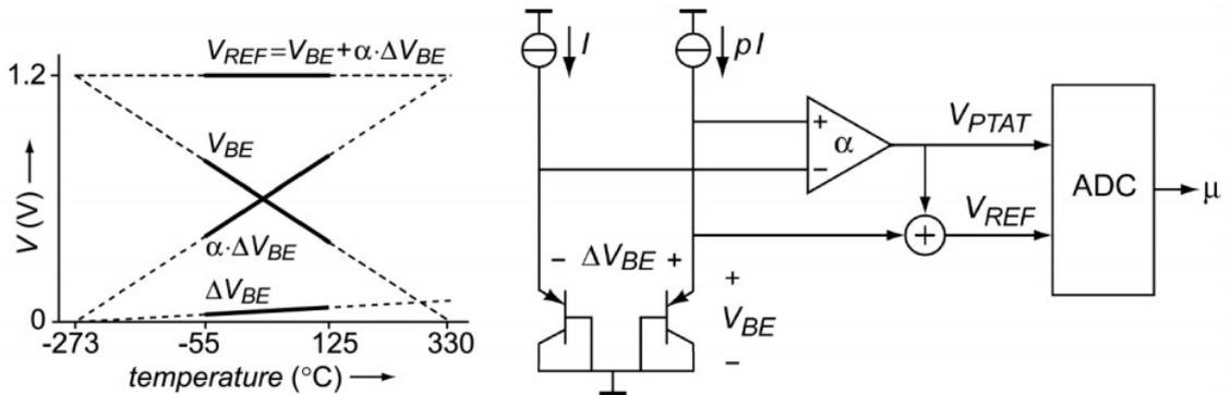
Figure 1.1: Block diagram of a BJT-based temperature sensor showing the generation of  $V_{be}$ ,  $\Delta V_{be}$ , and  $V_{ref}$  [10]
