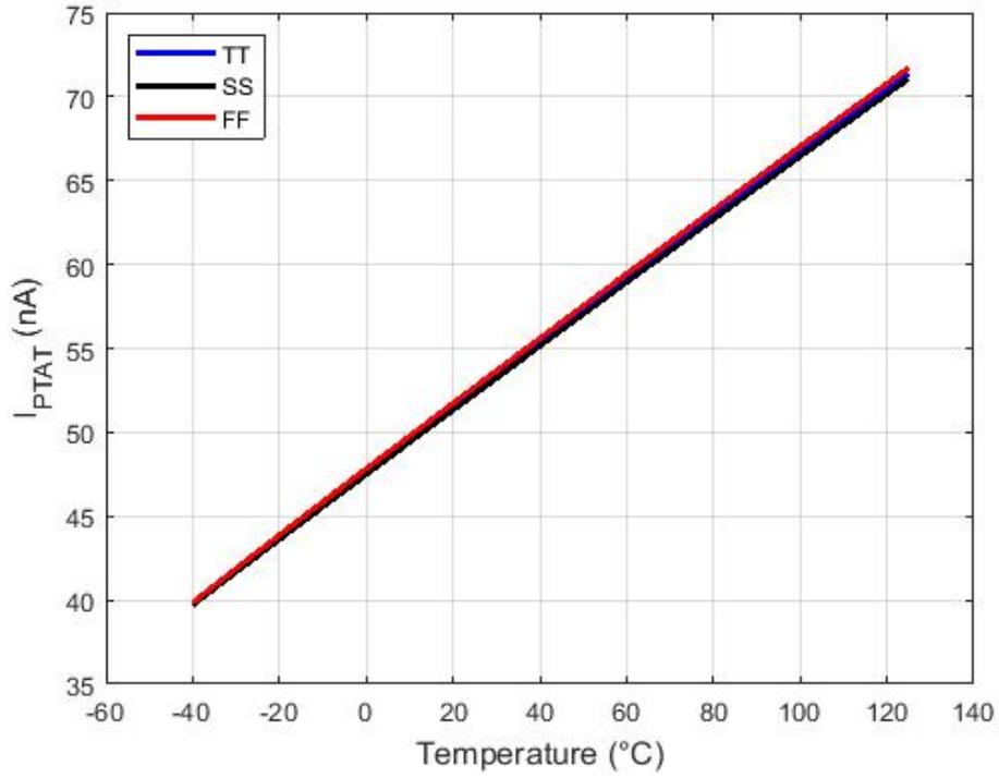
Figure 3.4:  $I_{PTAT}$  current across the temperature at different process corners
