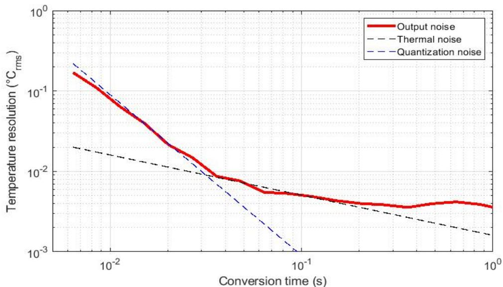
Figure 5.5: Temperature resolution (°C) across the conversion time (s)
