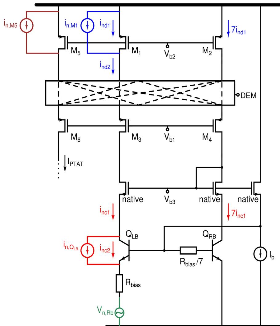
Figure 3.10: Schematic of the PTAT current generator with the dominant white-noise sources annotated (the white-noise sources of  $Q_{RB}$  and  $M_2$  are not shown for simplicity)
