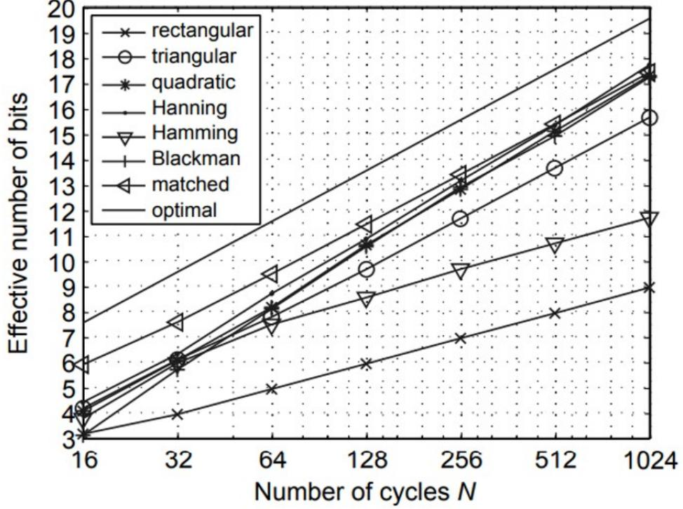
Figure 2.2: Second-order  $\Delta\Sigma$  modulator: ENOB versus the number of clock cycles [10]
