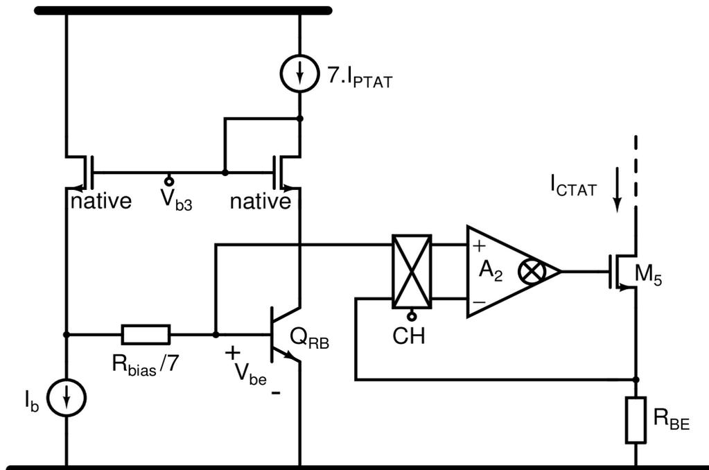
Figure 3.6: Schematic of the CTAT current generator
