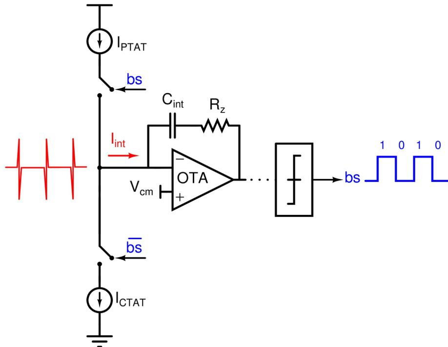
Figure 4.5: Simplified schematic for the  $\Delta\Sigma$  modulator showing the switching transients of  $I_{int}$
