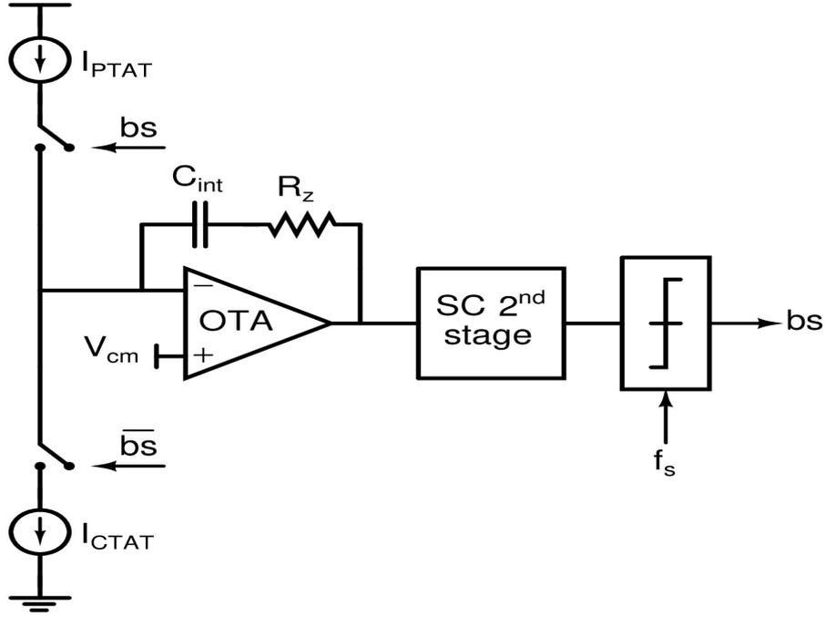
Figure 4.2: Schematic showing the 1<sup>st</sup> integrator of the  $\Delta\Sigma$  modulator
