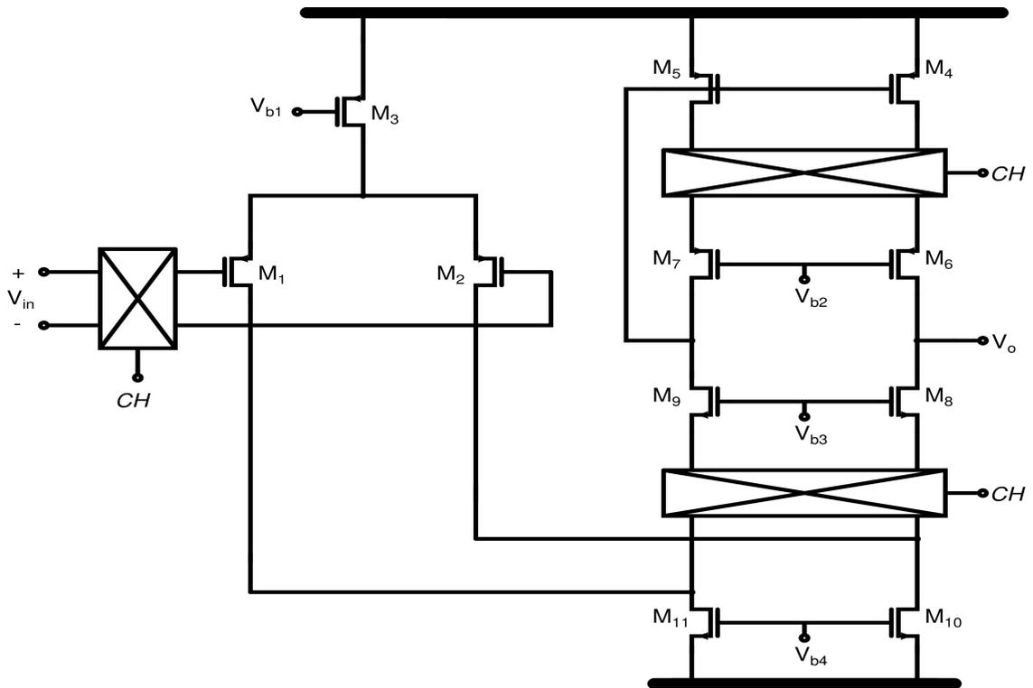
Figure 3.7: Schematic of the chopper folded-cascode OTA  $A_2$  in the CTAT current generator
