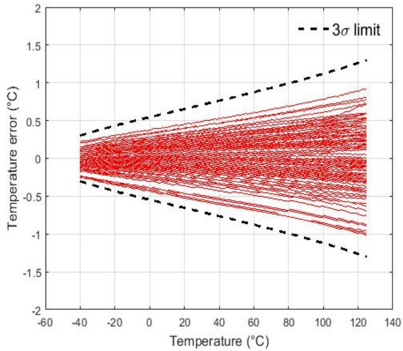
Figure 5.2: MC simulation: residual temperature error after systematic non-linearity removal
