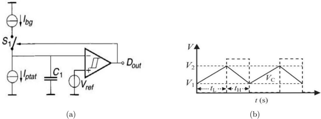
Figure 1.2: Schematic diagram showing the concept of duty-cycle modulation in temperature-sensing. (a) Basic principle (b) the voltage across  $C_1$  [8]
