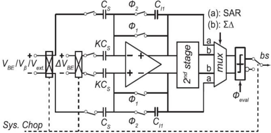
Figure 1.5: Two-step TDC showing the scaled sampling capacitors [2]
