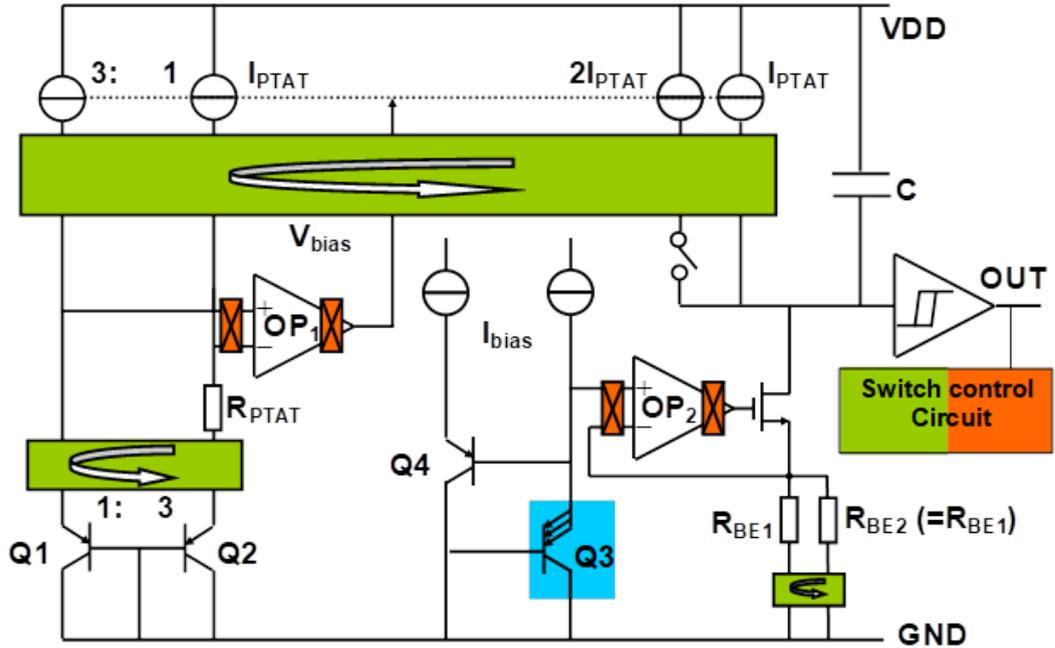
Figure 1.3: Circuit schematic of BJT-based temperature sensor with duty-cycle modulated output [8]
