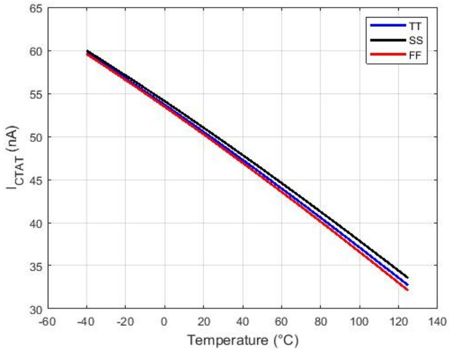
Figure 3.8:  $I_{CTAT}$  current across the temperature at different process corners
