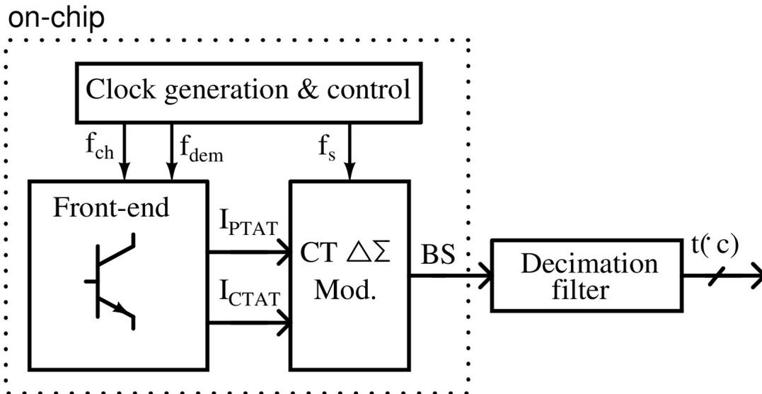
Figure 2.1: Block diagram of the BJT-based TDC with continuous-time  $\Delta\Sigma$  modulator
