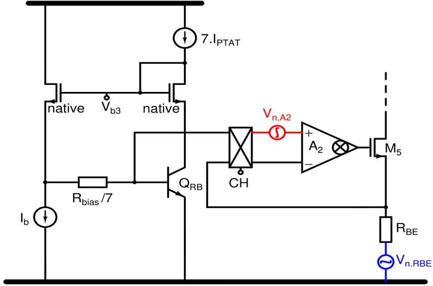
Figure 3.11: Schematic of the CTAT current generator with the dominant white-noise sources annotated
