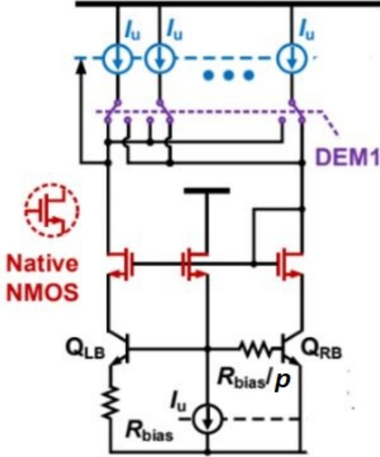
Figure 3.1: Schematic of NPN-based PTAT current generator [13]
