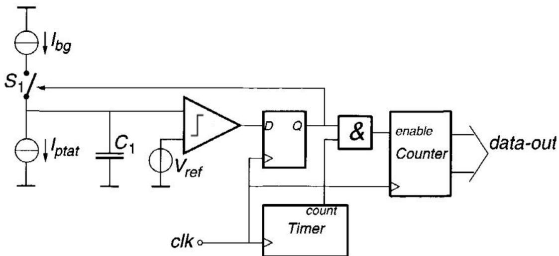
Figure 1.4: Block diagram showing the principle of the  $\Delta\Sigma$  modulator in BJT-based temperature sensor [28]
