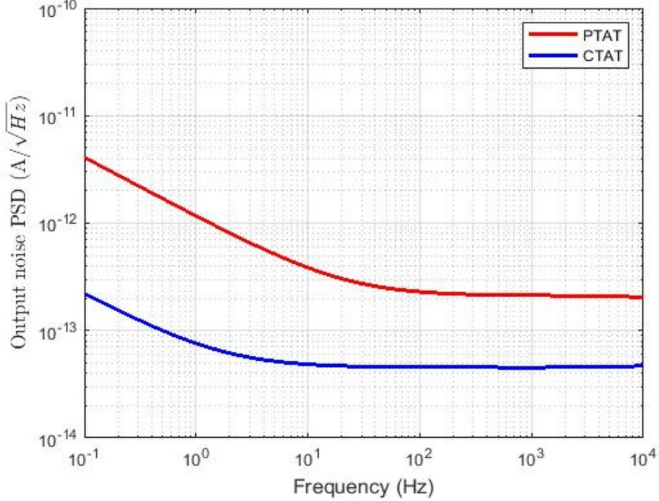
Figure 3.12: Simulated output noise current PSD ( $A/\sqrt{Hz}$ ) associated with  $I_{PTAT}$  and  $I_{CTAT}$
