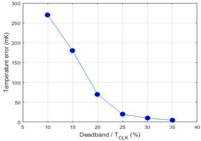
Figure 4.7: Simulated temperature error across the deadband percentage of the sampling clock period
