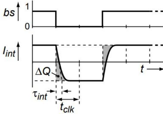
Figure 4.6: switching transients in the integrated current  $I_{int}$  lead to inter-symbol interference [10]
