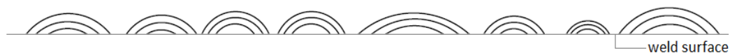
Figure 4. 28: Assumption of multiple crack initiation at crack coalescence stage in the surface of the weld
