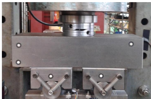
Figure 3. 5: Fixture and rollers of the upper side of the 4PB specimen
