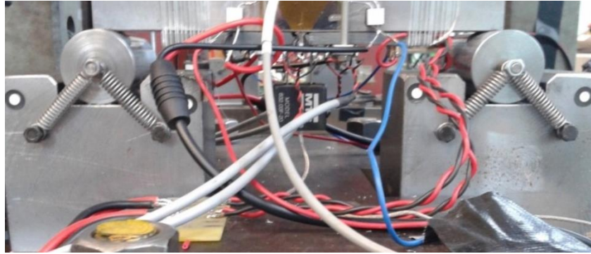
Figure 3. 6: Fixture and rollers of the lower side of the 4PB specimen
