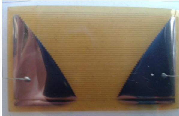
Figure 3. 10: Crack gauge consists of 40 grid lines with spacing 0.50 mm
