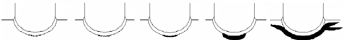
Figure 1. 3: Crack propagation on a tubular T-joint
