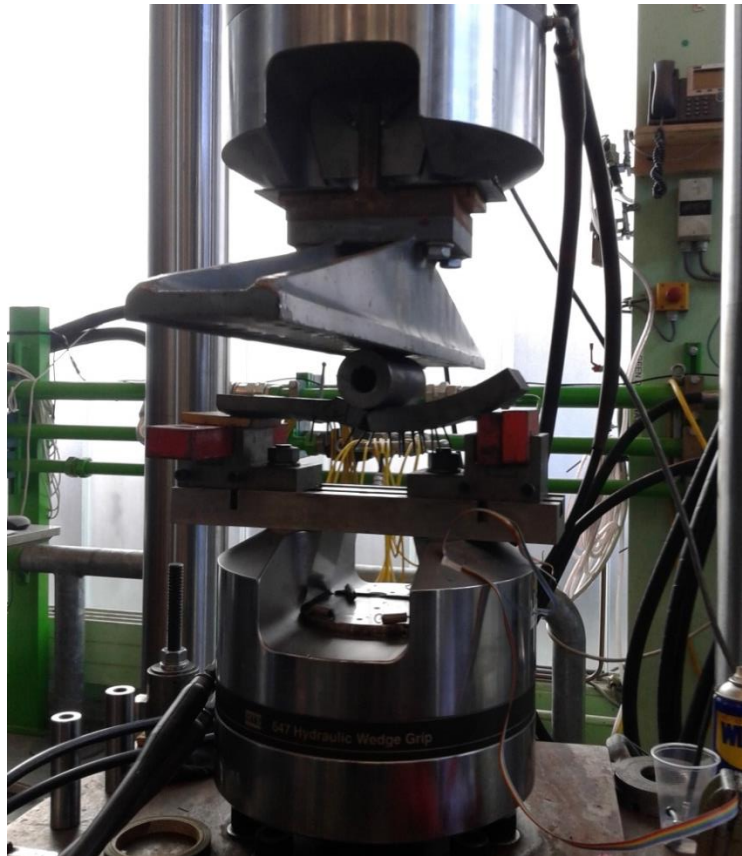
Figure 4. 34: 3-point bending test on a slice of the tubular joint
