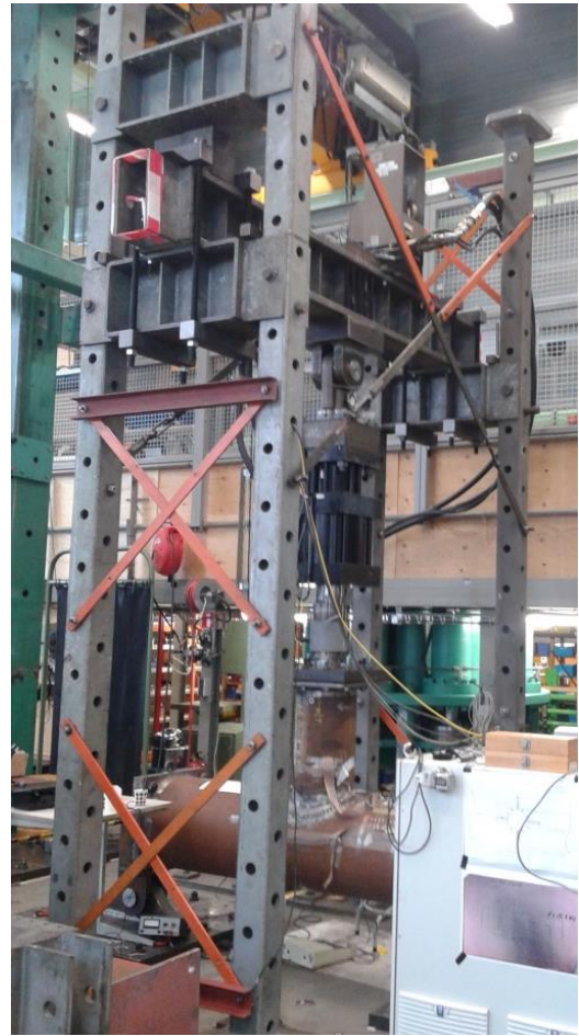
Figure 4. 5: The servo-hydraulic actuator and the test rig of the experiment
