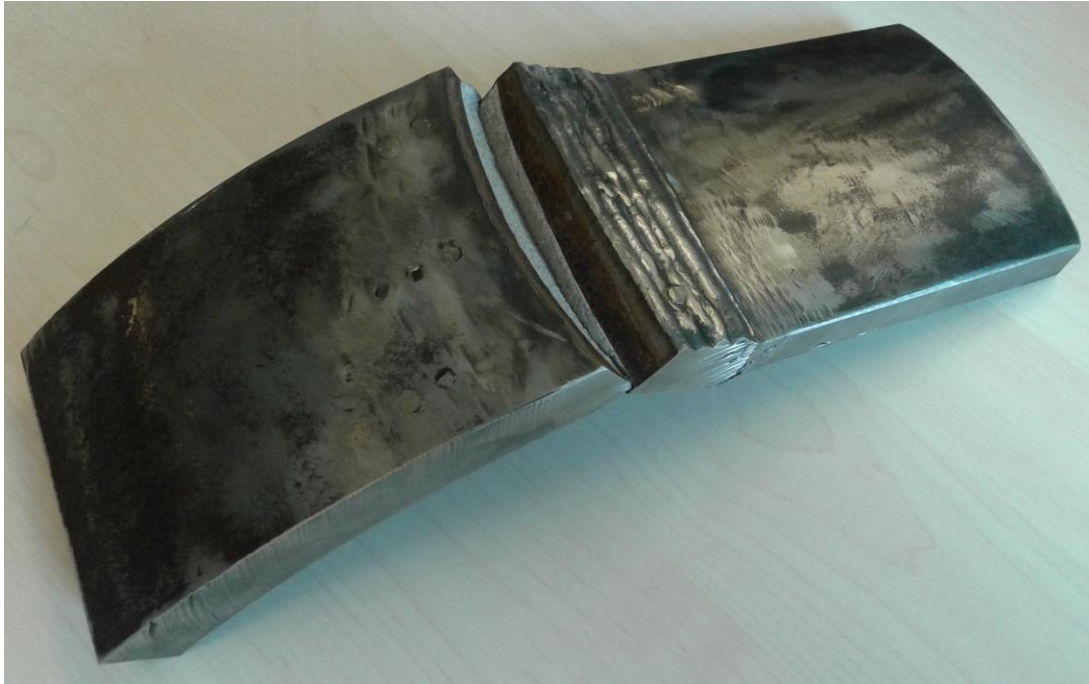
Figure 4. 35: Opened crack on a slice of tubular joint
