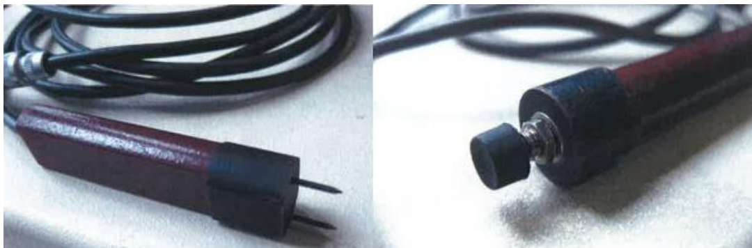
Figure 4. 12: Probe used for voltage measurements
