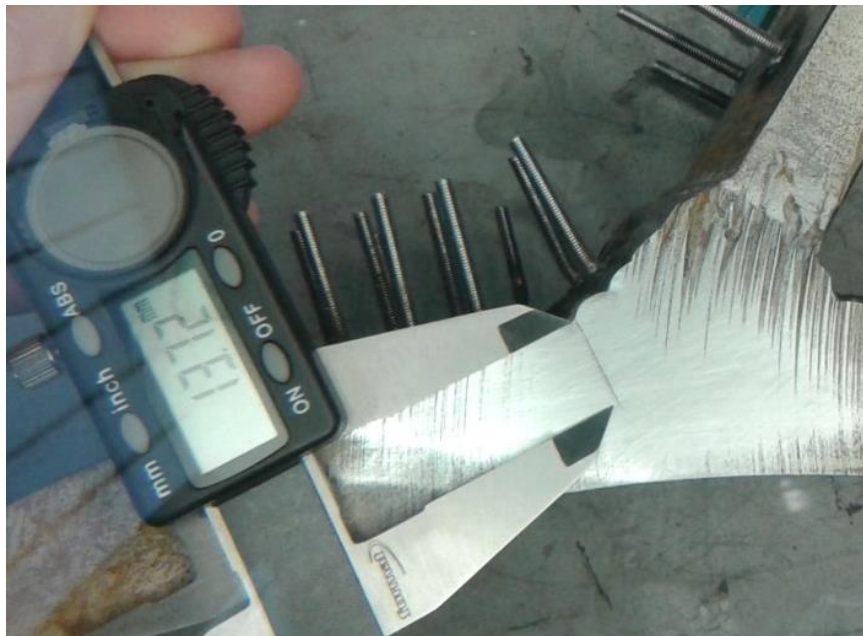
Figure 4. 33: Measuring through thickness crack
