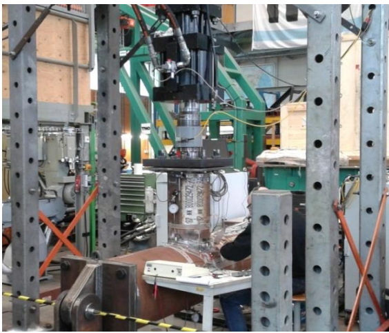
Figure 4. 5: The servo-hydraulic actuator and the test rig of the experiment
