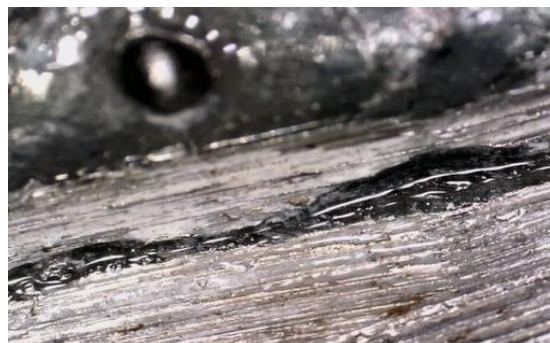
Figure 4. 8: Crack length determination via microcamera
