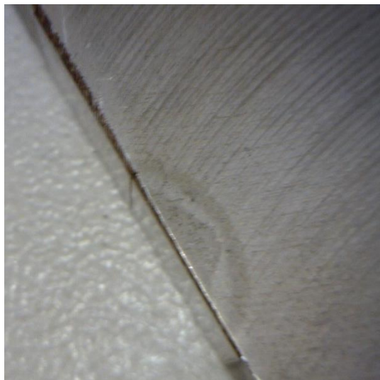
Figure A. 2: Bead weld on plate heat affected zone
