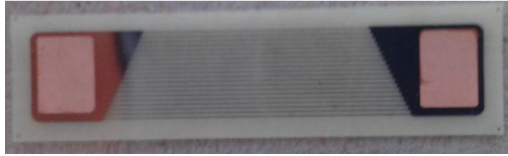
Figure 3. 9: Crack gauge consists of 20 grid lines with spacing 0.25 mm
