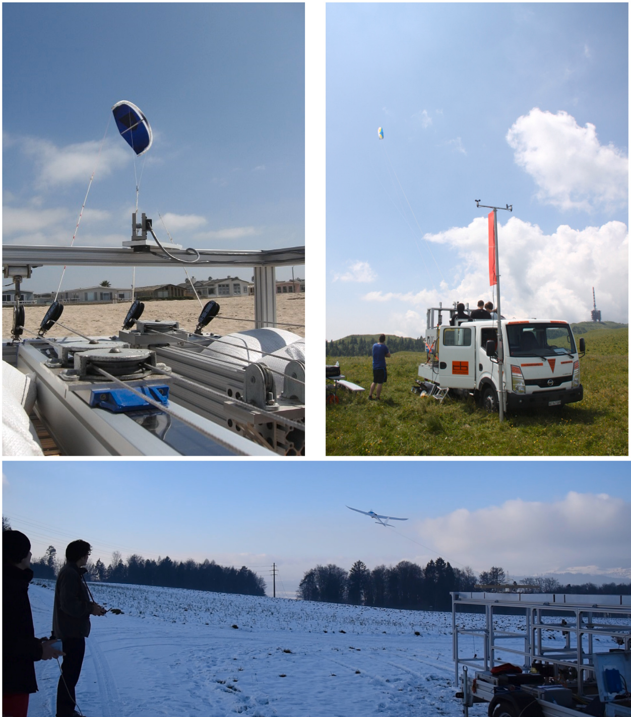
Fig. 29. Examples of prototypes for field tests whose results and data are available to the research and development community. Clockwise from top left: UCSB prototype (Fagiano & Marks, 2015; Fagiano et al., 2014), Swiss Kite Power prototype (Zgraggen et al., 2016), ABB Corp. Res. prototype (Fagiano et al., 2017, 2018).
