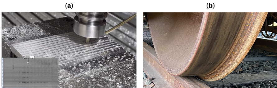
Figure 2.5: (a) Marks on the machined surfaces due to chatter. Image credit: Richconn; (b) Steel railway wheel in contact with a steel rail. Image credit: Gary T. Fry / Railway Age.
