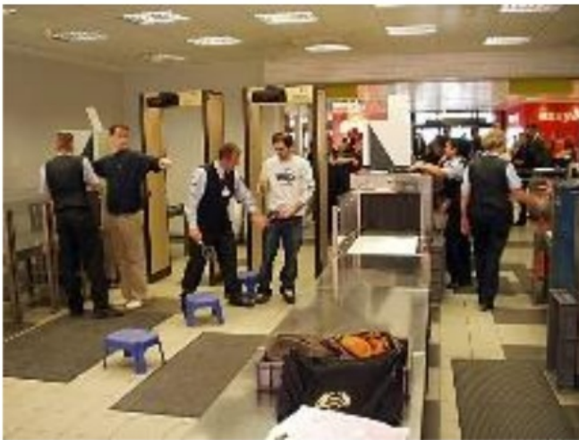
Figure 2. Combination of x-ray scanner and metal detector, for luggage and travelers respectively. (Davies, 2012)
