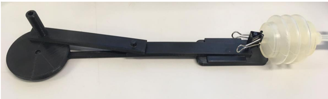
Figure 56: Slider and crank mechanism was 3D printed in polycarbonate to automatically actuate the test lung.
