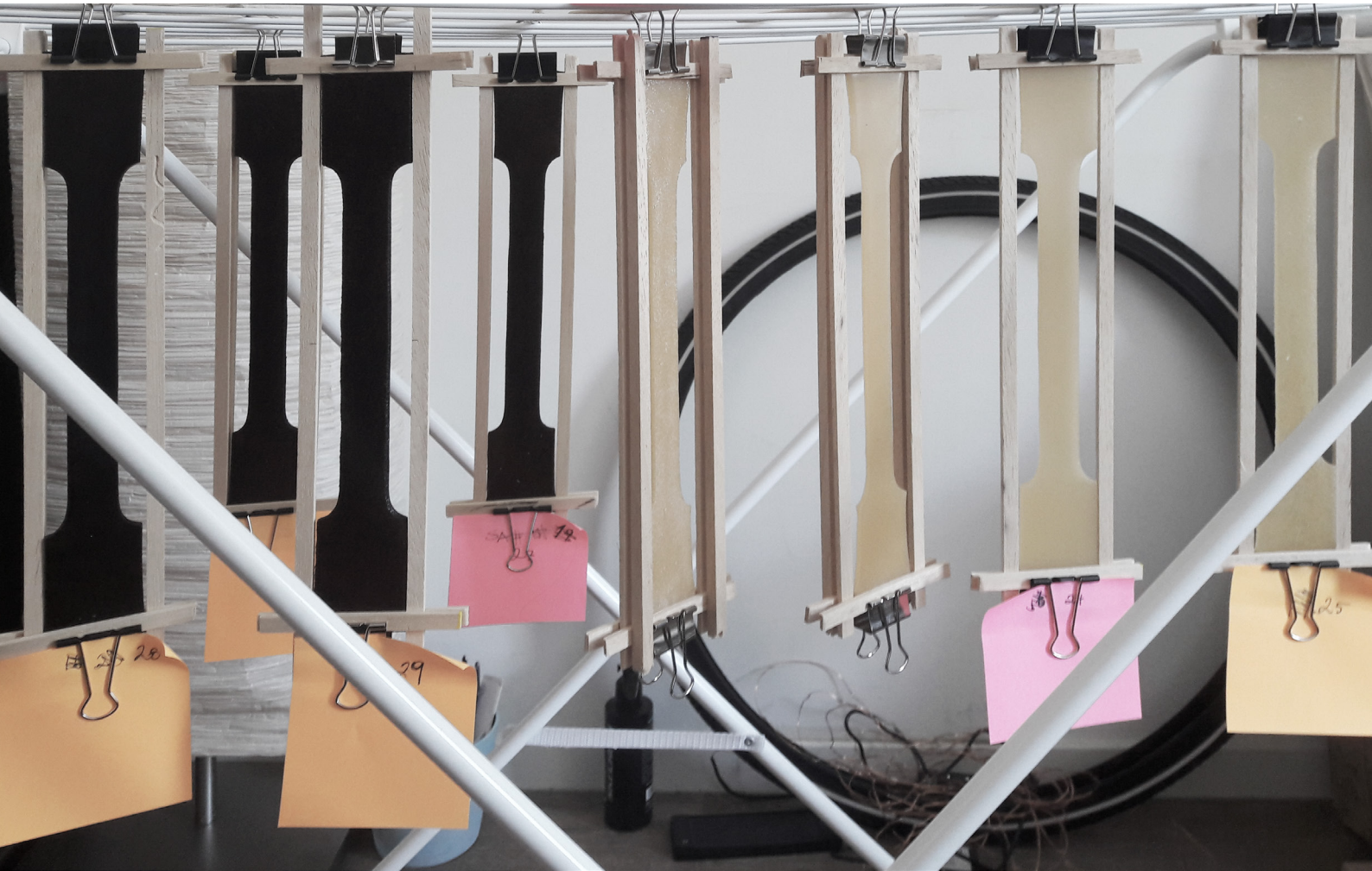
Figure 3.5: Some of the specimens as they are drying and curing in the frames.
