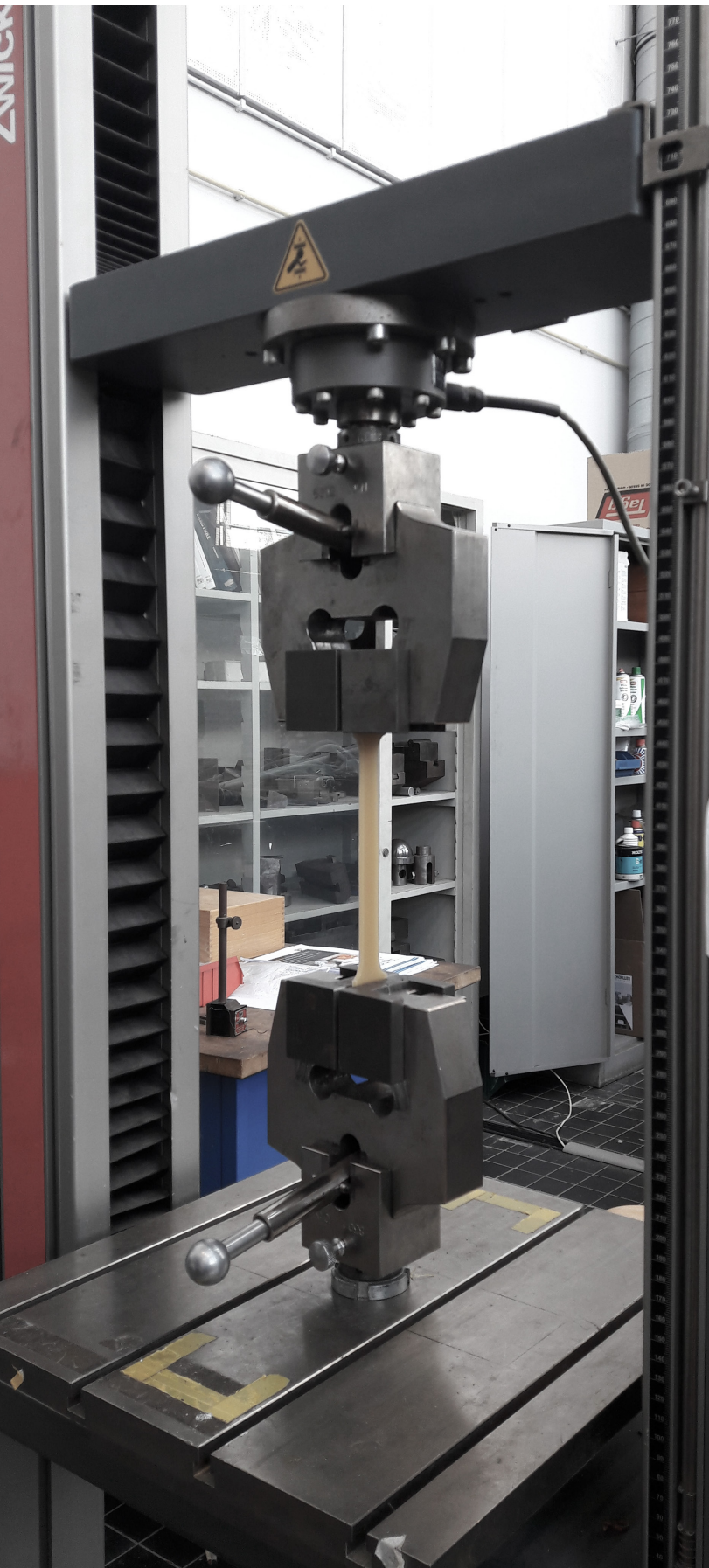
Figure 3.10: Tensile strength test at 3mE TU Delft
