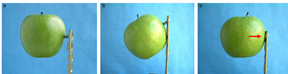
Figure 2.21: Visualization of the advantage of locking screws by Cronier et al [10]. Figure (A) With a locking screw, the assembly is stable. (B) With an untightened common screw, the assembly is unstable. (C) Compression is necessary against the plate. From [10]
