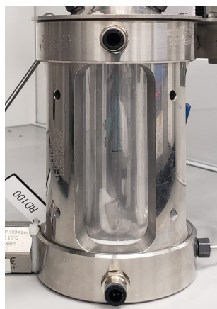
Figure 3.4: Sapphire Visualization Cell: A transparent and durable setup for visual observation of dynamic phenomena in closed systems. The SVC including housing has a diameter of 10 cm and height of 15 cm.
