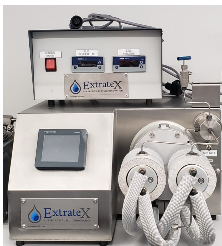
Figure 3.6: Volumetric \text{CO}_2 Pump Used to Attain Critical \text{CO}_2 Pressure for the Experiments. The pump is 50 cm x 45 cm x 25 cm.
