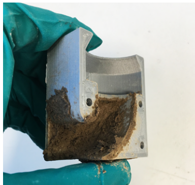
Figure 4.9: The stiff material got stuck in the nozzle during the waiting period of the open time test, which is one of the reasons to restrict the printed amount.
