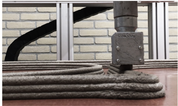
Figure 3.4: A lab-scale 3DCP configuration at TU Delft: (a) 3D CNC table and material conveying pump; (b) Down-flow nozzle with a round opening ( \varnothing 15 mm).
