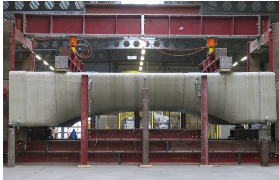
Figure 8.5: The test setup for large-scale 3D printed structural elements in TU Eindhoven, adapted from [38].
