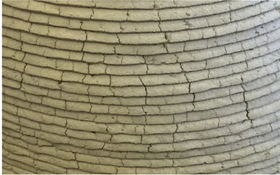
Figure 8.2: Drying plastic shrinkage induced cracks on the printed cementitious materials, adapted from [3].
