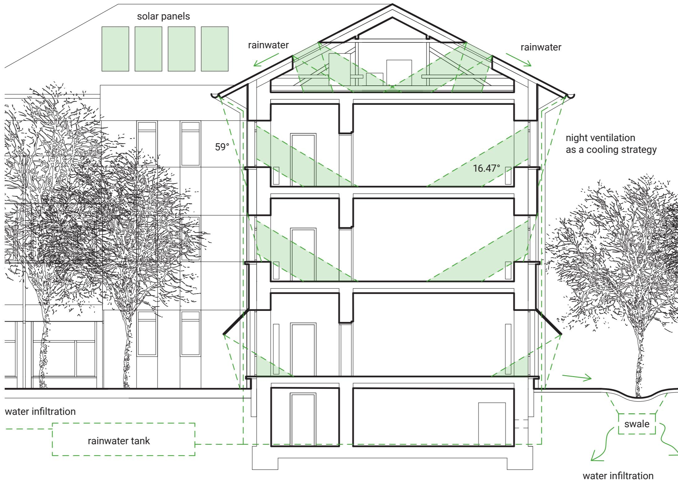
rainwater collection, shading, solar gains, cooling
