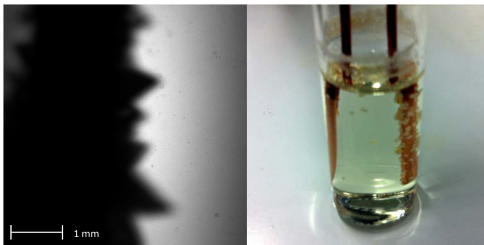
Figure 8-3. Left: Slightly out of focus faceted crystals growing on the surface of the anode in the presence of the inhomogeneous electric field. Right: Crystals on the anode in a vial after a solution crystallization in the presence of an electric field strength of 5.6 \times 10^5 \text{ V m}^{-1} (initial solution concentration of 35 \text{ mg mL}^{-1} , a cooling rate 1 \text{ }^\circ\text{C min}^{-1} ).
