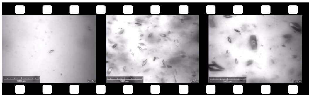
Figure 2-6. Crystal growth of RDX visualized with the Crystalline Particle Viewer. The crystal size rapidly increases with the time.
