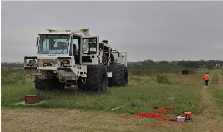
Figure 1.3: Vibroseis source truck. Picture taken by Dr. Rik Noorlandt.
