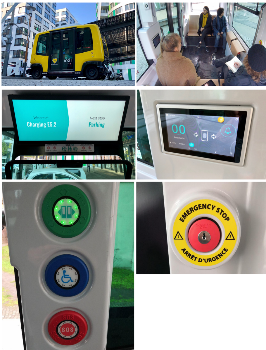
Fig. 1. A (top left) Automated shuttle ‘Emily’ by Easymile on the EUREF campus in Berlin B (top, right) Accompanied test ride with two respondents (front), the interviewer and steward hidden as minute writer C (middle, left) Information display with route information D (middle, right) Operator interface E (below, left) Door opening button (top), button to pull out wheelchair ramp (middle), button to connect the shuttle to an external control room (below) (not active when test rides were performed) F (below, right) Emergency stop button.
