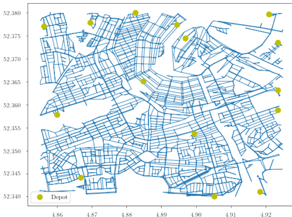
Figure 5.9: Depot distribution using the K-center Method: 15 depots are placed throughout the graph and are represented by the yellow indicators.
