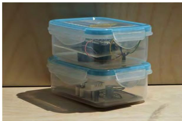
Figure 2.5.4: Second casing solution with the boards inside, but still missing the ventilation openings, sun-reflective foil and the tie-wraps for securing to the vehicle (own work)
