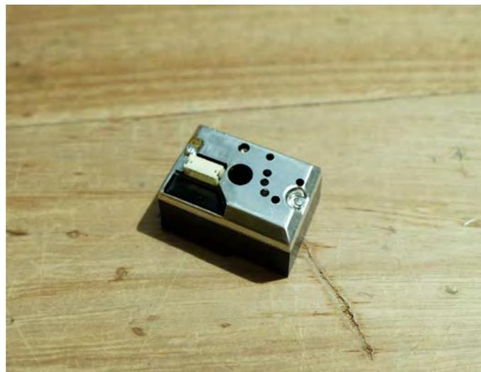
Figure 2.4.5: The dust sensor GP2Y1010AU0F (own work)
