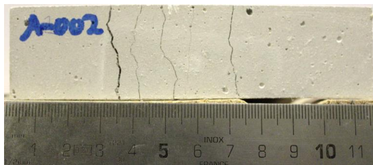
Figure 4.9 Crack pattern of specimen A-002 after loading.
