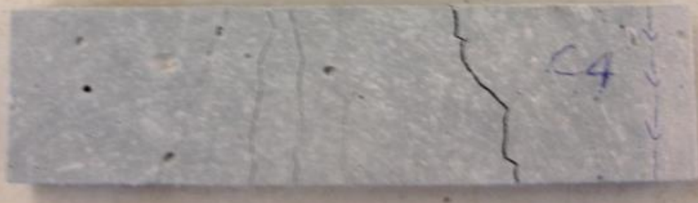
App. E - Figure 3 Crack Pattern of specimens C.
