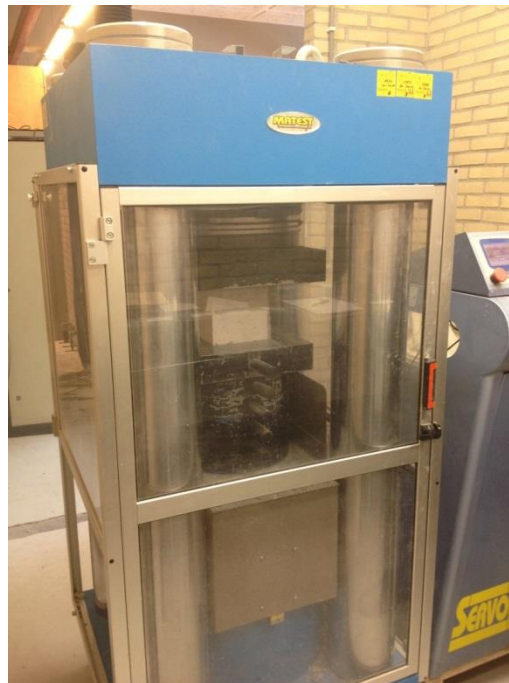
Figure 5.5 Test setup for the cube compression test in chapter 5.
