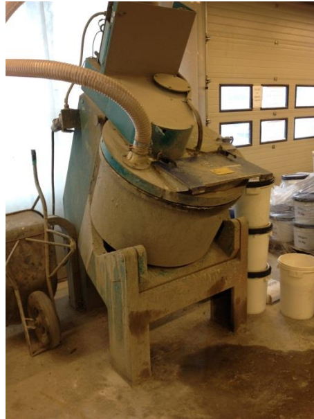
Figure 5.6 Mixing equipment for large scale production of SHCC.
