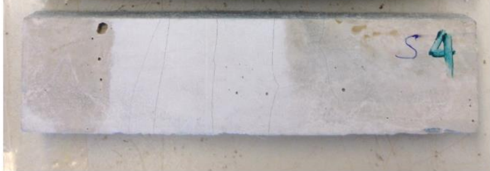
App. E - Figure 4 Crack Pattern of specimen ML specimens batch 2.
