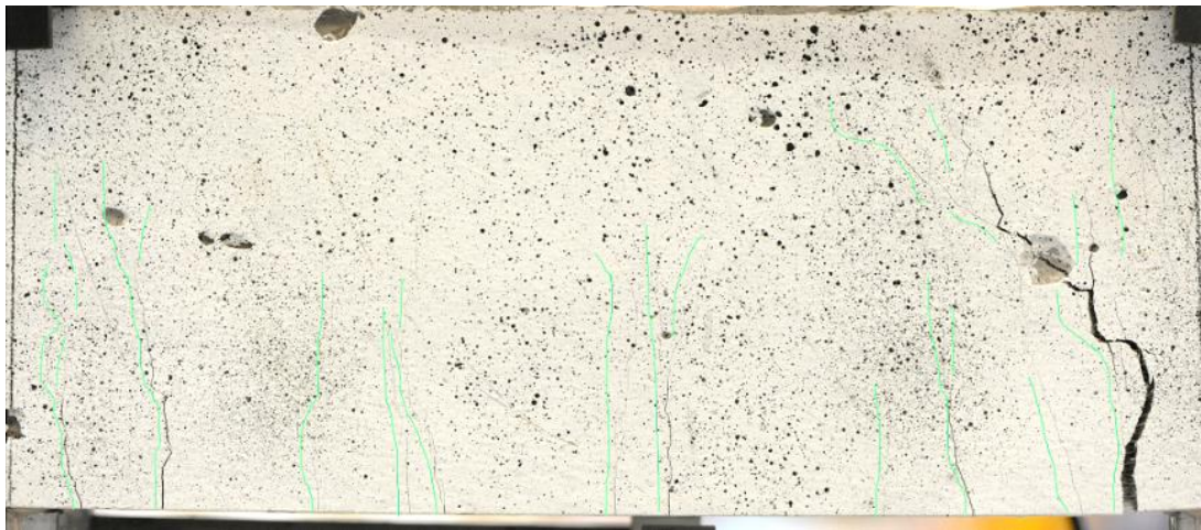
Figure 5.26 The displacement versus the pixel location (upper) for specimen FM700-002, and corresponding picture of analyzed area with cracks highlighted with green lines (lower).
