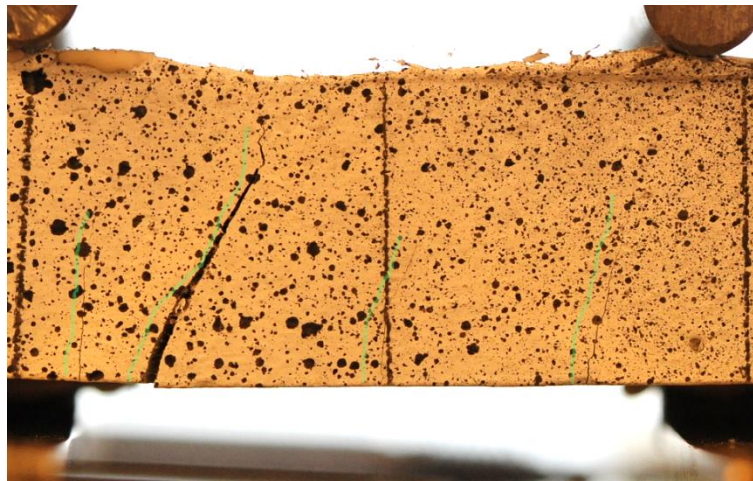
Figure 5.24 The displacement versus the pixel location (upper) for specimen FM175-001, and corresponding picture with cracks highlighted with green lines (lower).
