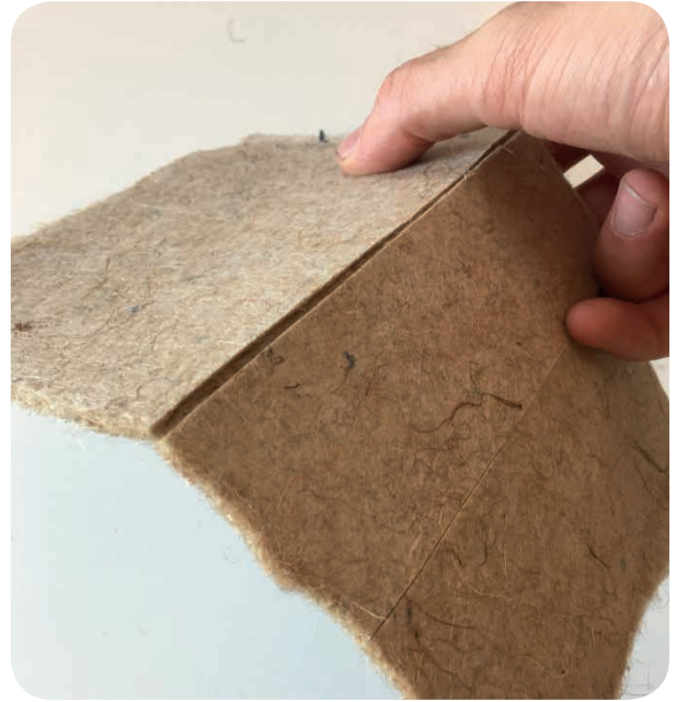
Fold 2. Engraved fold figure 49. An engraved fold. By cutting the upper half of a fold line, a fold is made.
