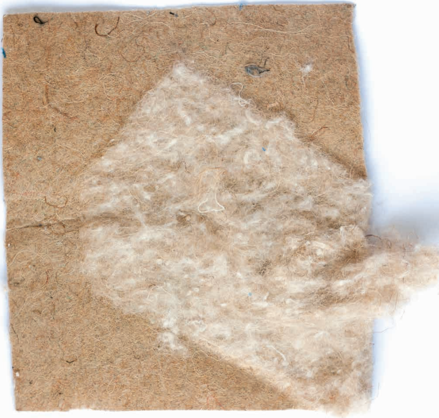
Figure 62. Sample heated with iron. This makes it possible to quickly make hard and soft areas locally. Heated areas hardly have any stiffnes
