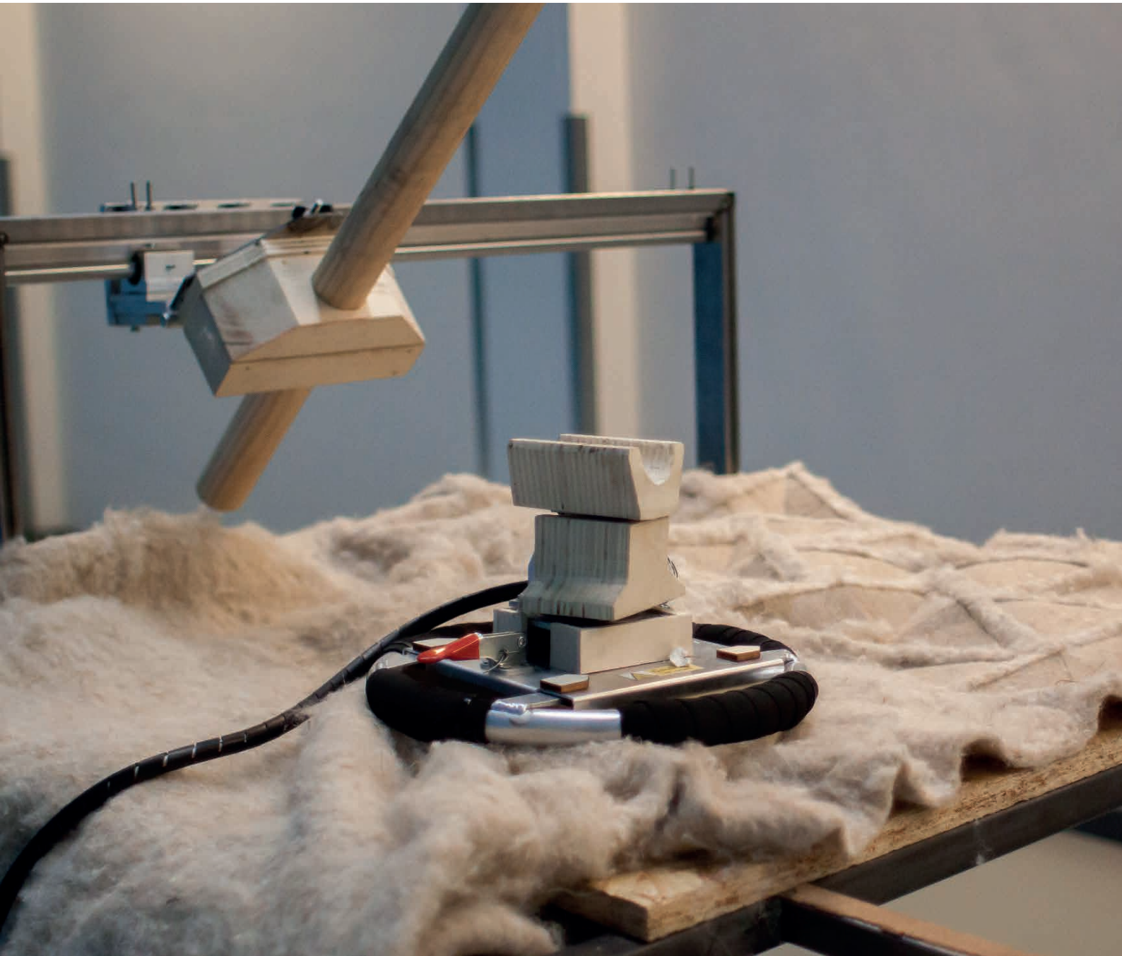
Figure 139. The heating unit on a piece of RECURF
