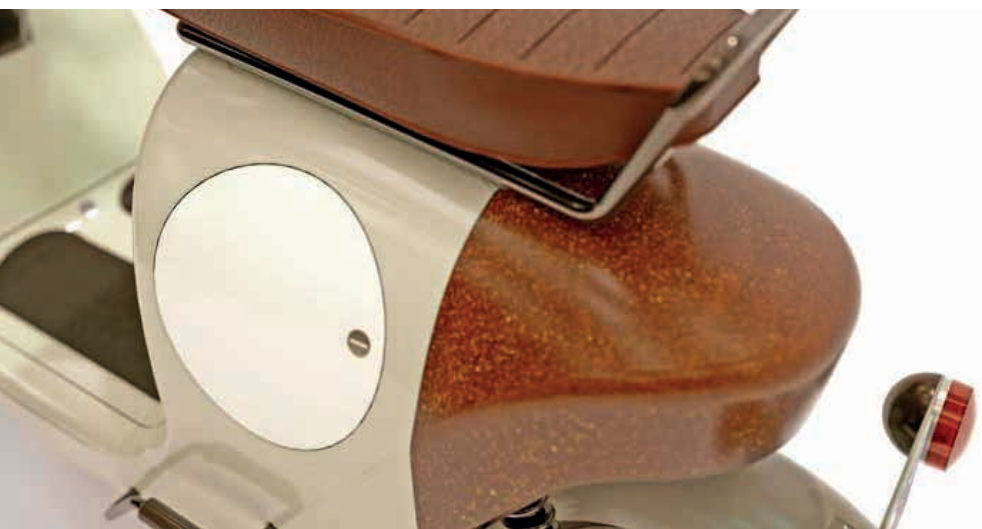
Figure 16. Scooter panel made of hemp fibers and bio resin. Be.e by Waarmakers [6]
