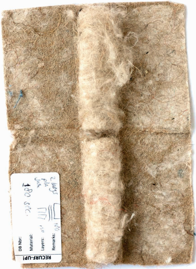
Figure 73. A soft fold made with the heat press. This soft fold also has an invisible fold going through its middle. This kind of intersection of folds is unpractical, because only one fold can be folded at a time.
