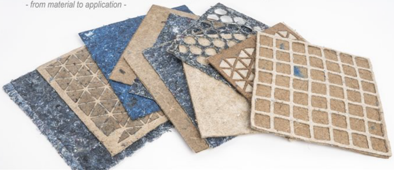
An example of the composite RECURF. The difference in color between the sheets is due to the use of other kinds of fiber
