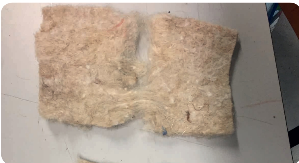
Figure 47. A soft sheet is Burlap RECURF can be torn in two by hand.
