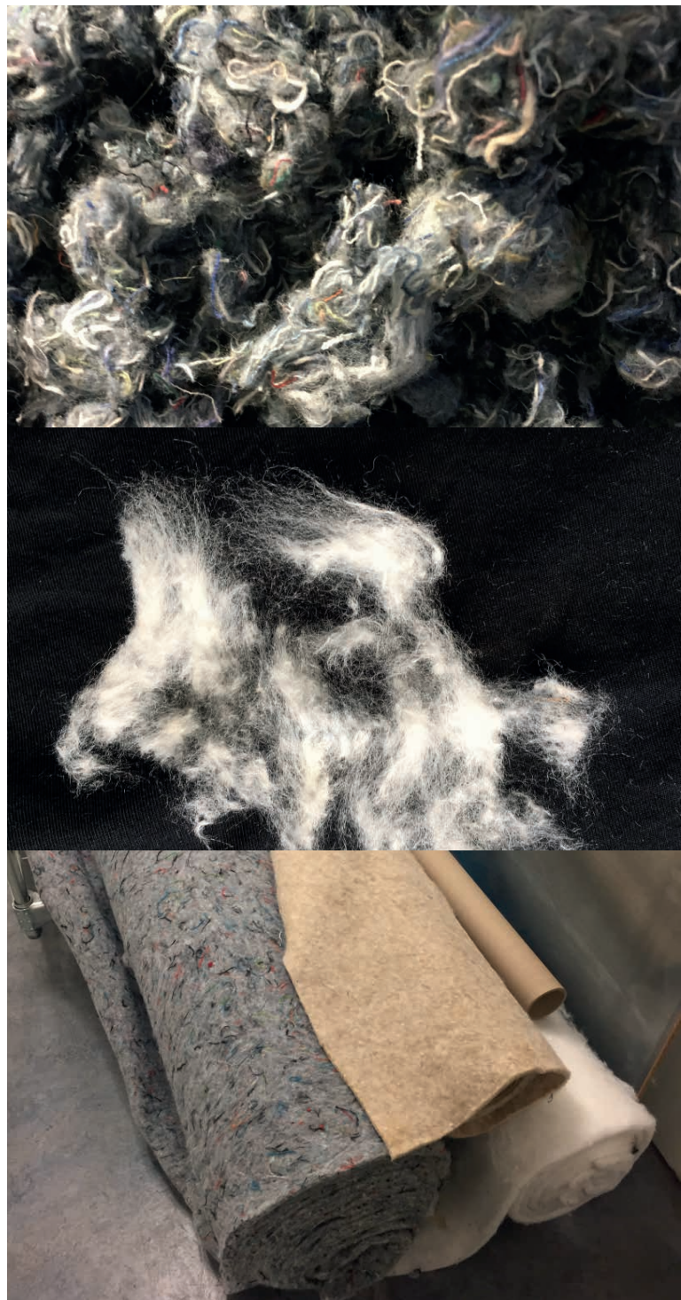
Figure 7. Top to bottom: A, B and C. A shows the denim fibers, B shows the PLA fibers. C shows the non-woven of the combination of denim and PLA.
