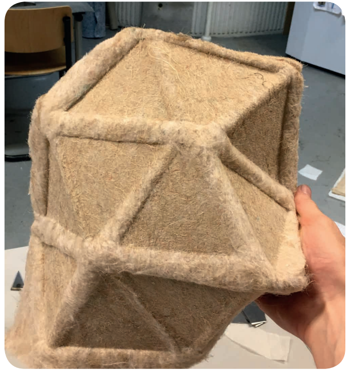
Figure 75. Invisible fold made of burlap PLA. Folding area made with the use of the flexibility of a single layer. Surrounding area is 3 layers thick.
