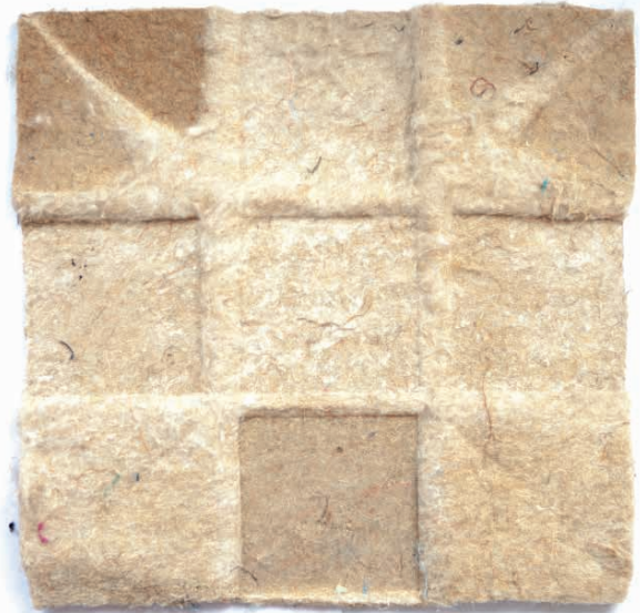
Figure 79. These origami patterns did not turn out as expected. They all had issues. Most were because of restrictions created by the use of the heat press.
