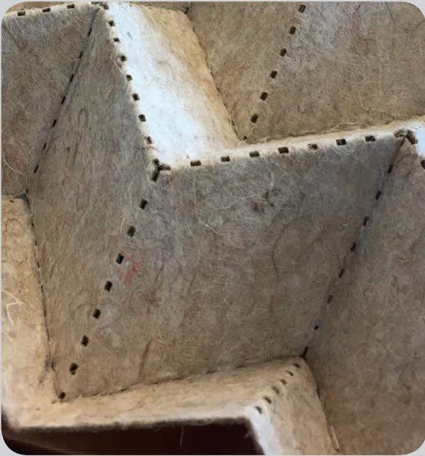
Fold 1. Dotted fold figure 48. Sample made by Ties Westerhuis. Example of a laser cut fold on BiCo material. One of the 6 kinds of folds explored during this session.
