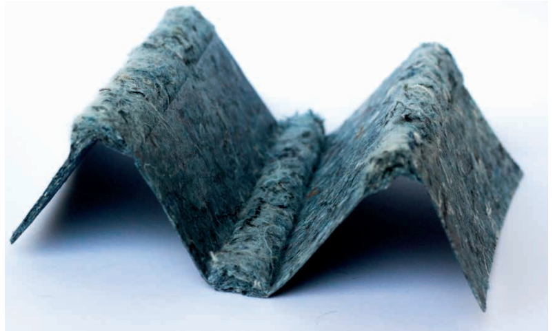
Figure 74. This sample has 2 soft fold next to each other. It can be noticed that when this fold is closed, only soft material is shown. Moving the origami means changing the contrast of the duality in hard and soft.
