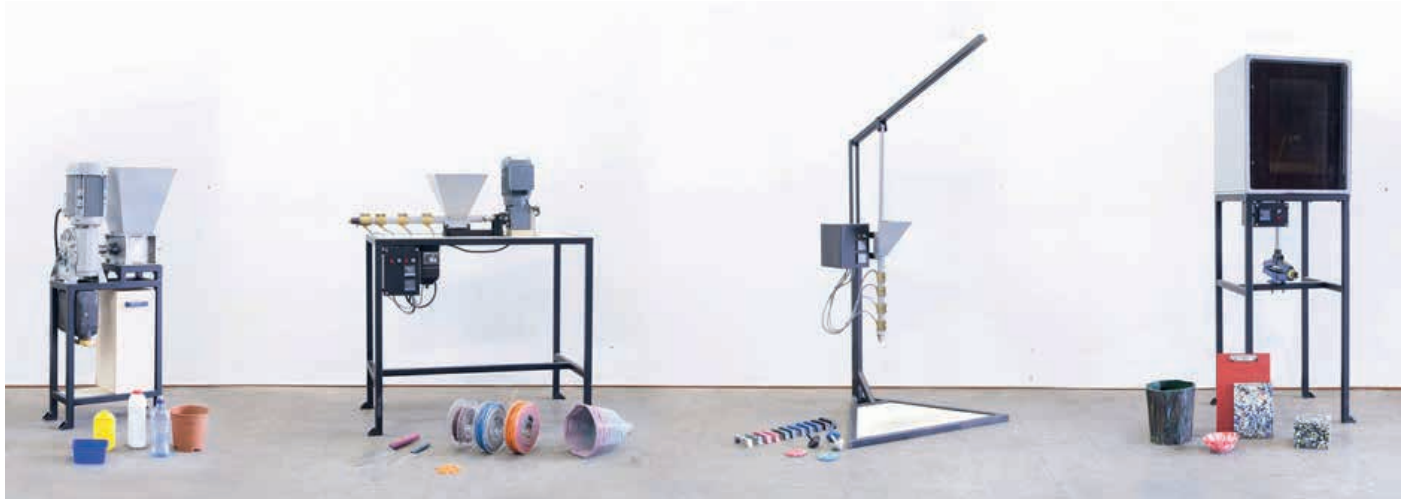
Figure 115. Plastic recycling machines by Dave Hakkens [37]
