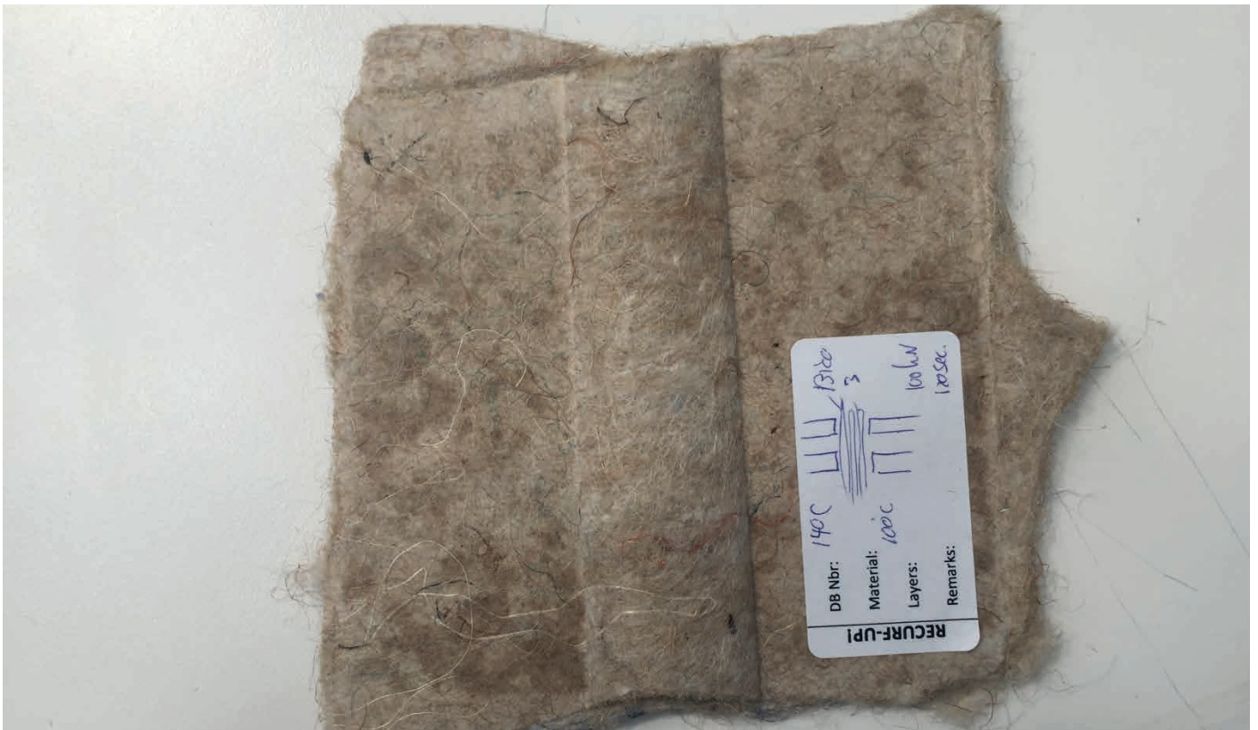
Figure 143. Dark spots visible. Often caused by high forces
