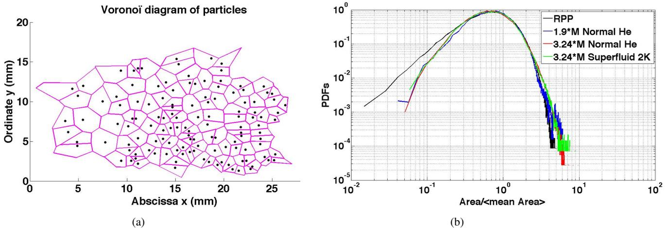
Figure 2. (a) example of Voronoi tessellation. (b) Probability distribution of normalized Voronoi area. RPP refers to Random Poisson Process. These measurements were taken at 5Hz.  $\frac{S}{M} = .83$  with S the stroke of the grid and M the mesh size. Their mean density  $\rho_{particles}$  is  $180\text{kg/m}^3$  and  $\rho_{Helium} = f(T) = (135 \pm 10)\text{kg/m}^3$ .
