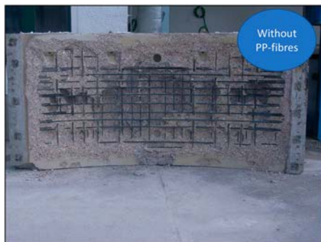
Fig. 5: Fire resistance design for the Amsterdam North/South metro line involved full-scale fire testing of tunnel lining segments, showing the effectiveness of adding polypropylene (PP) fibres to the concrete mixture in largely mitigating the spalling sensitivity (based on project documents)
