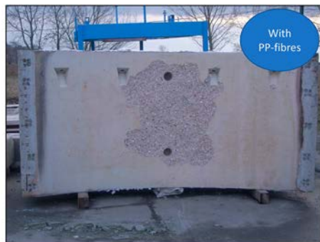
Fig. 5: Fire resistance design for the Amsterdam North/South metro line involved full-scale fire testing of tunnel lining segments, showing the effectiveness of adding polypropylene (PP) fibres to the concrete mixture in largely mitigating the spalling sensitivity (based on project documents)
