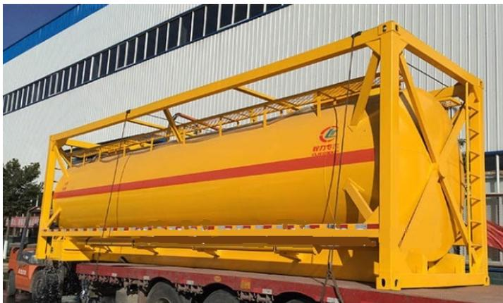
Figure 3.19: Fuel oil/gasoline tanktainer [6]
