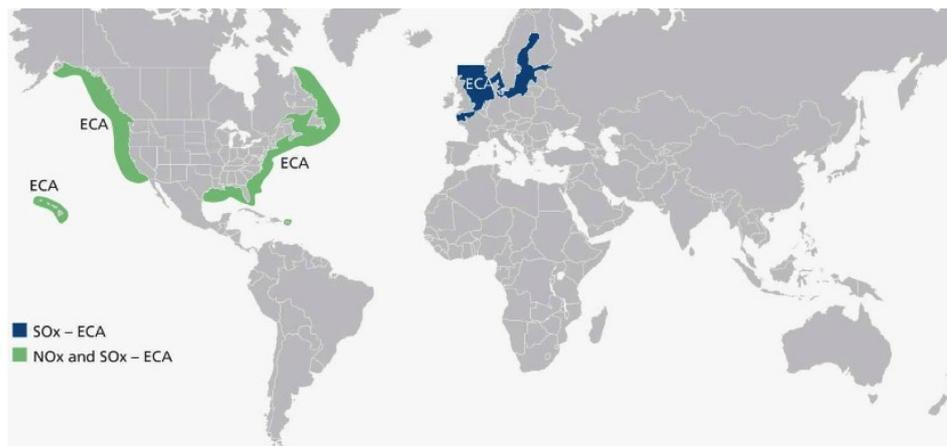
Figure 2.1: Current SO<sub>x</sub> and NO<sub>x</sub> ECAs [51]
