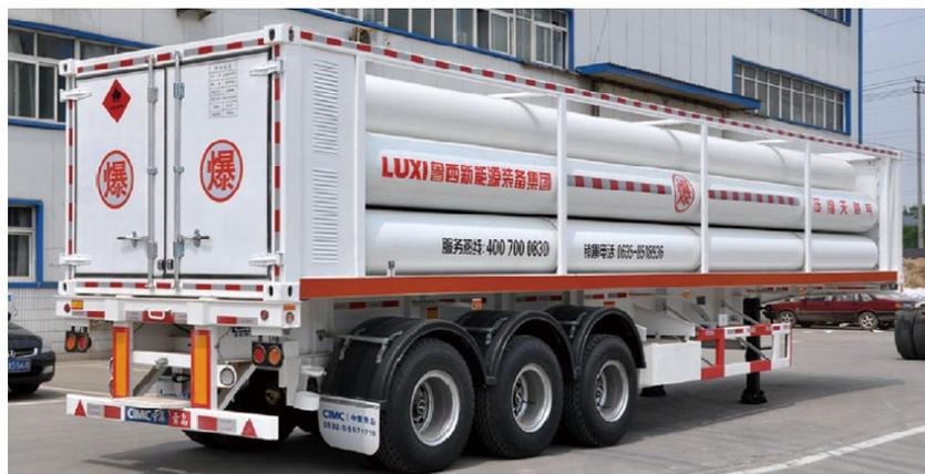
Figure 3.16: Tube skid container [57]
