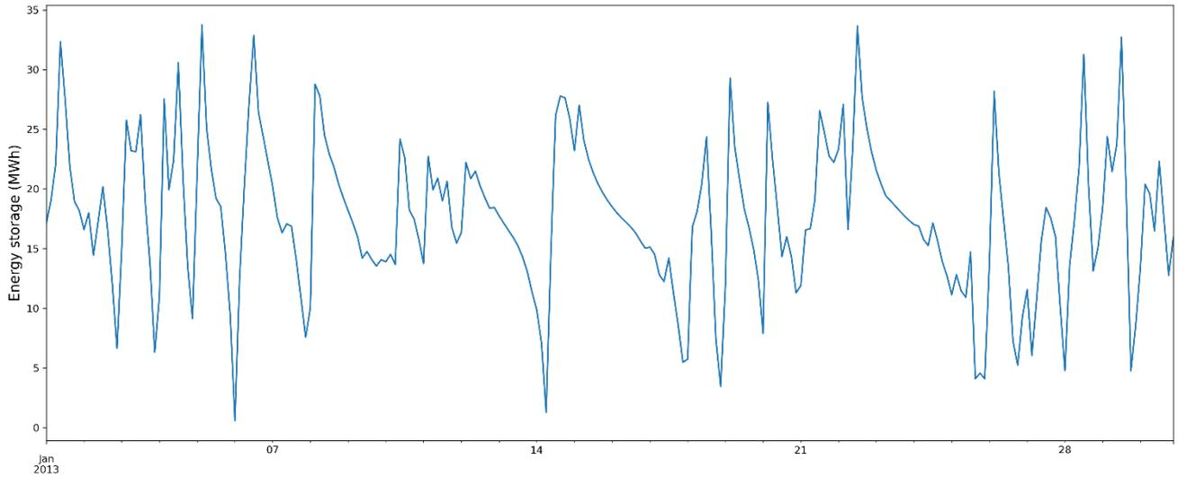
Figure 27: modeled state of charge of battery energy storage in January 2013 in the baseline scenario.
