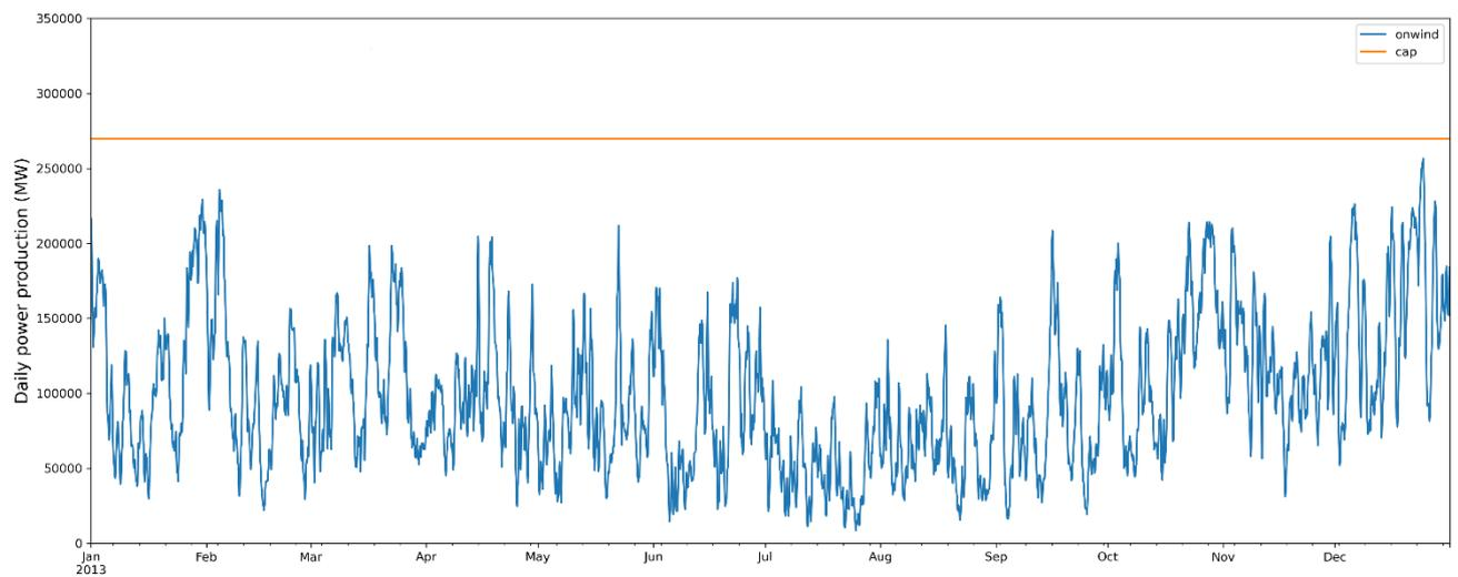
Figure 19: modeled aggregated onshore wind electricity generation in the North Sea countries in the baseline scenario. The horizontal orange line denotes the onshore wind power capacity.
