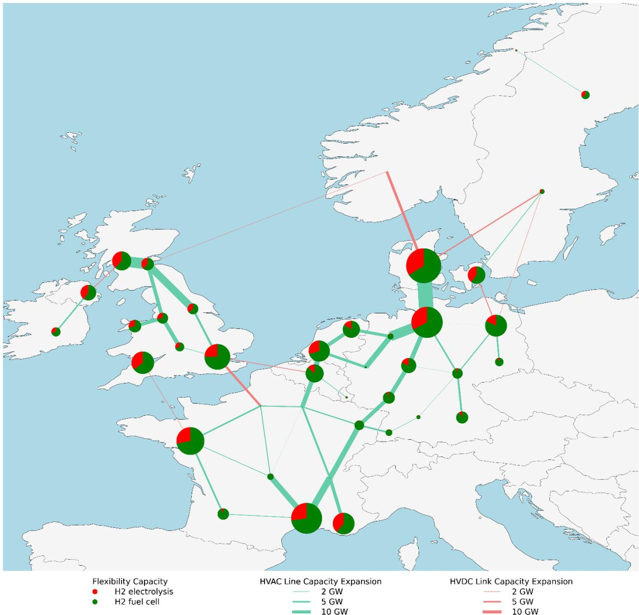
Figure 10: hydrogen electrolysis capacity, hydrogen fuel cell capacity, and the transmission network expansion of the baseline scenario.
