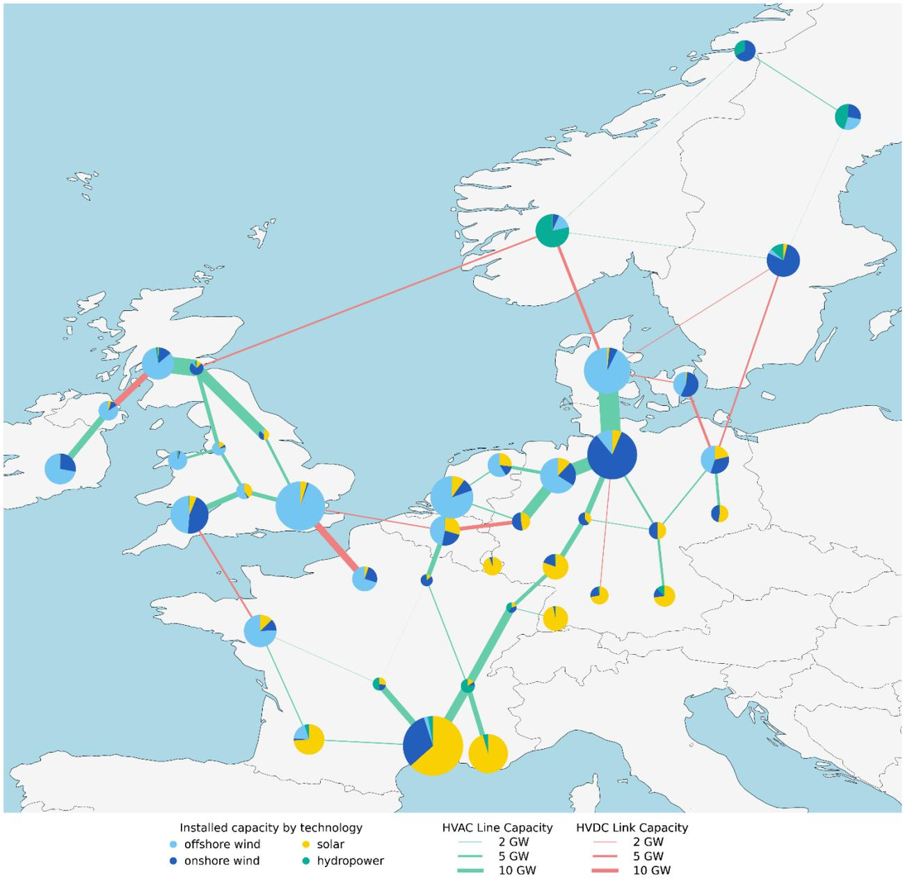
Figure 17: lay-out of the transmission network of scenario 13. In scenario 13, tank storage is used to store hydrogen instead of salt caverns.
