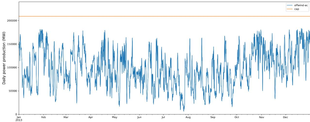
Figure 20: modeled aggregated offshore wind electricity generation connected by AC lines in the North Sea countries in the baseline scenario. The horizontal orange line denotes the offshore wind capacity installed via an alternating current connection line.
