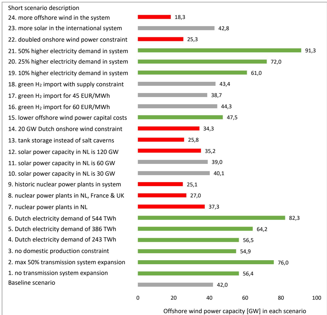
Figure 9: overview of offshore wind power capacities in each scenario. An increase in offshore wind capacity of more than 10% relative to the baseline scenario is coloured in green, a decrease of more than 10% is coloured red and a change of less than 10% relative to the baseline scenario is coloured in grey. A comprehensive description of the scenarios is shown in Table 16.
