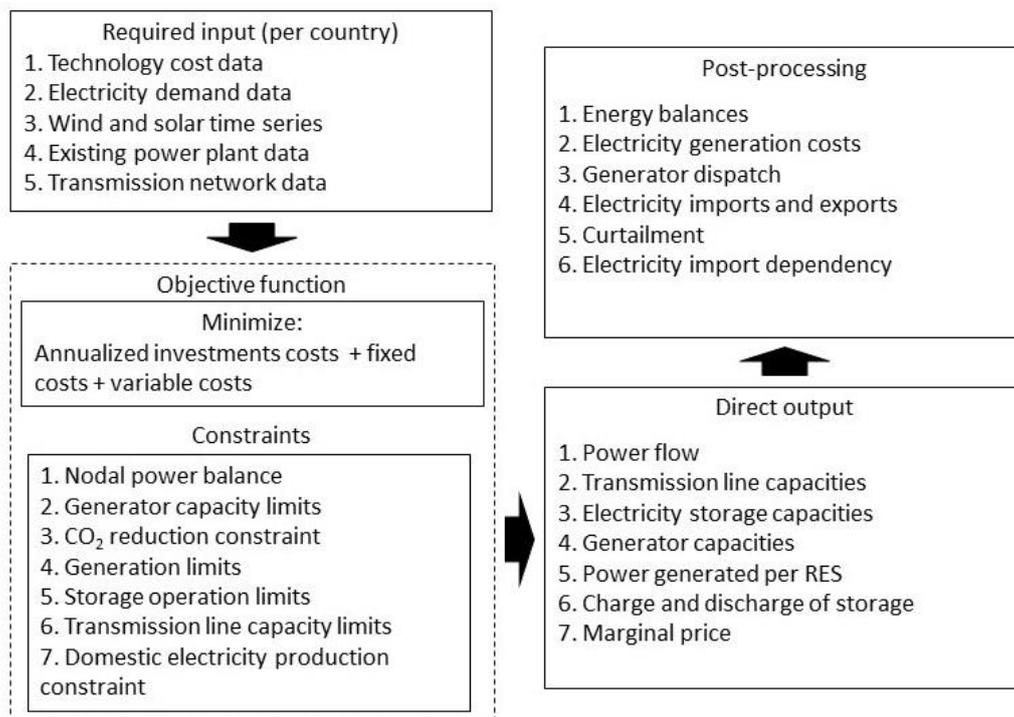
Figure 5: Methodological elements of the used model based on PyPSA-Eur.
