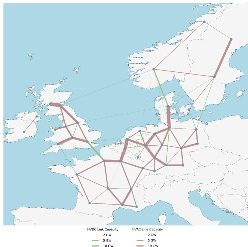
Figure 6: PyPSA-Eur model of the electricity system of the North Sea countries including all existing high-voltage alternating current (HVAC) and high-voltage direct current (HVDC) lines.
