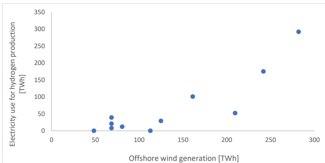
Figure 2: relation between offshore wind generation and green hydrogen production. A capacity factor of 46% for offshore wind capacity is assumed.
