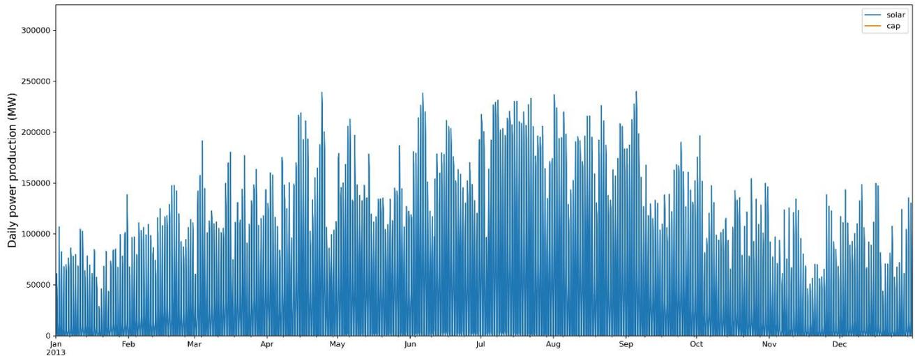
Figure 18: modeled aggregated solar PV electricity generation in the North Sea countries in the baseline scenario. The horizontal orange line denotes the solar PV capacity.
