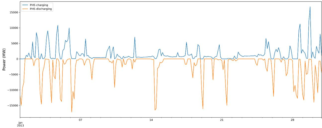
Figure 31: electricity generation and consumption of pumped-storage hydroelectricity in January 2013 in the baseline scenario.
