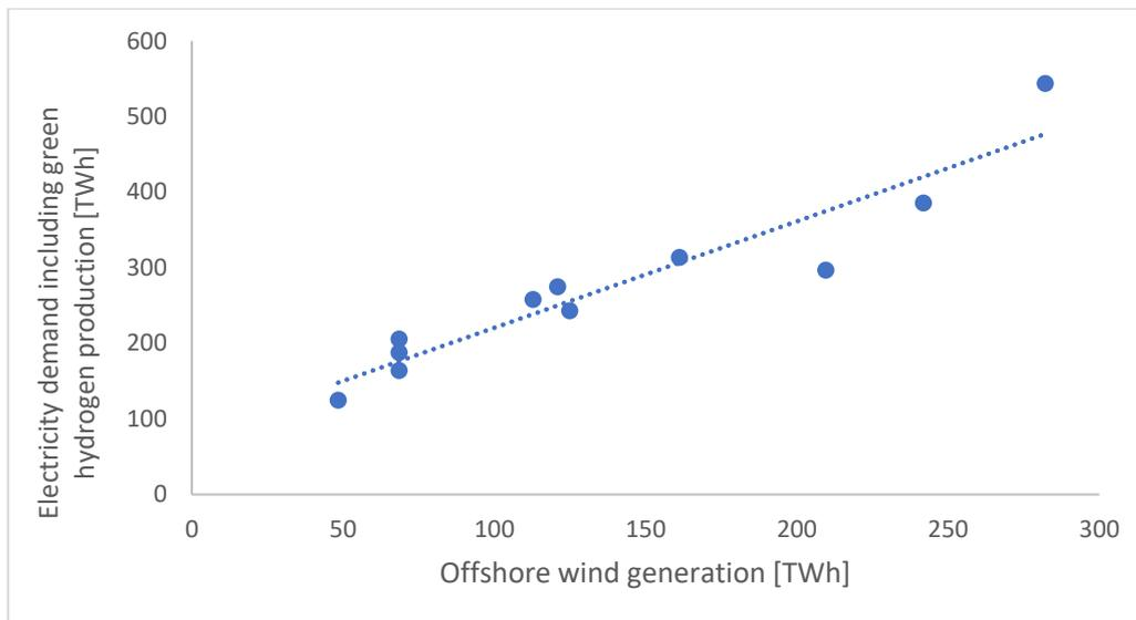
Figure 1: relation between offshore wind generation and electricity demand. A capacity factor of 46% for offshore wind capacity is assumed.
