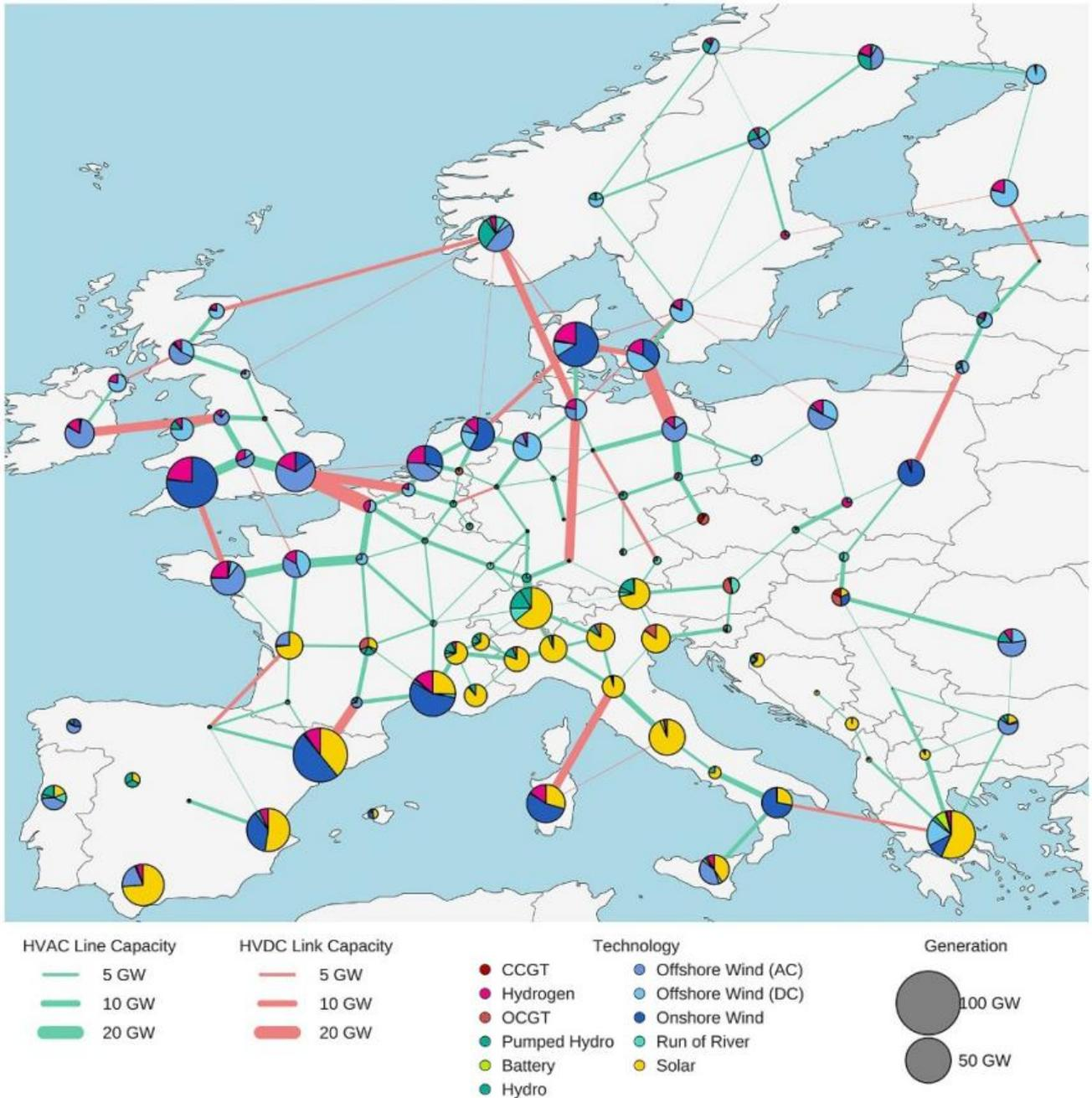
Figure 8: map of transmission line expansion, storage capacities, and power plant capacities per node in the optimal transmission network expansion with a 100% CO<sub>2</sub> reduction scenario in Neumann and Brown (2021).
