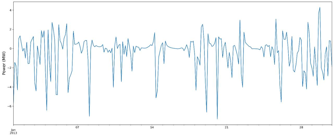
Figure 30: power charging and discharging of batteries in January 2013 in the baseline scenario.
