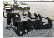
Figure 2.26: Quick Release Hook (QRH) arrangement on a mooring dolphin in Amsterdam (Straatman, 2020)
