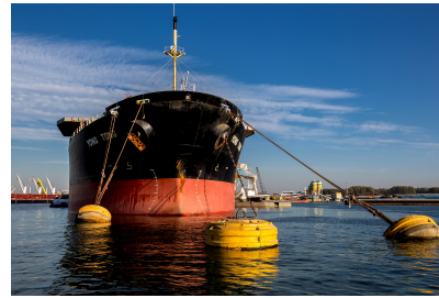
Figure 2.19: Mooring buoys in Port of Rotterdam (Port of Rotterdam, 2015)
