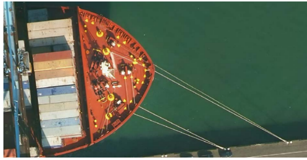
Figure 2.15: Forecandle deck with mooring lines and winches (Broos et al., 2018)
