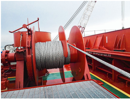
Figure 2.14: Winch with a split drum (Wilhelmsen, 2023)
