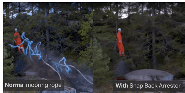
Figure 2.13: Comparison of mooring line snap-back with and without a snap-back arrestor. A regular mooring line recoils violently after breaking, while the mooring line equipped with a snap-back arrestor demonstrates a substantial reduction in recoil distance (Wilhelmsen, 2022).
