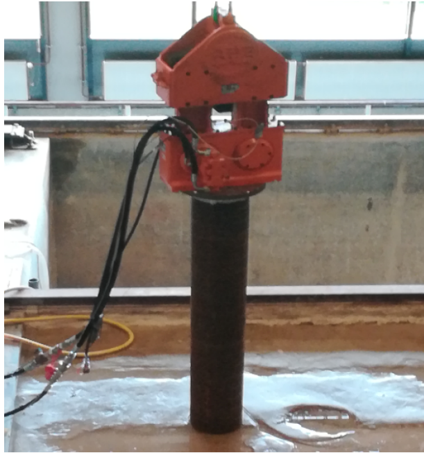
Figure 3.1: Experimental setup, showing the pile held by the crane and the pneumatic hammer.
