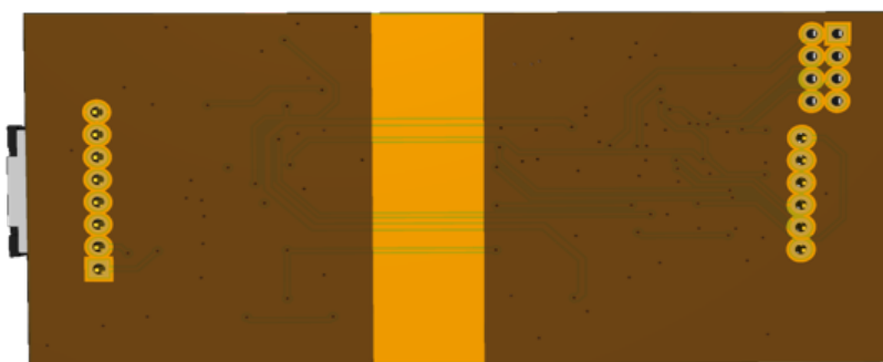
Figure 6.3: PCB Version 2 layout (back view with stiffeners).
