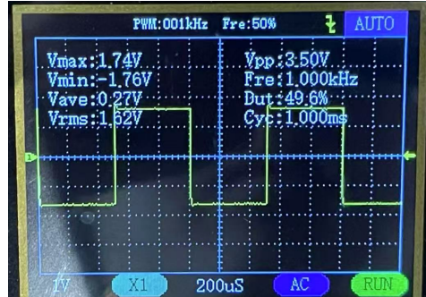
Figure 5.3: PWM in oscilloscope, 1 kHz
