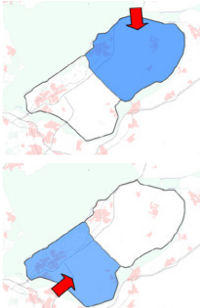
Figure 2.2.1: Compartmenting function of the Knardijk.
