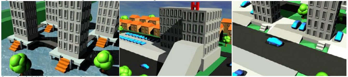
Figure 3.1.2: Building elevated: building elevated on poles, a non-livable ground floor, or a difference in level between street level and ground floor.
