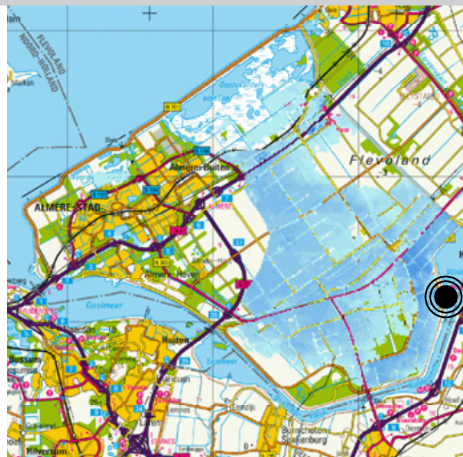
Figure 8.7.22: Max. water depth after breach near Zeewolde, alternative 1b.
