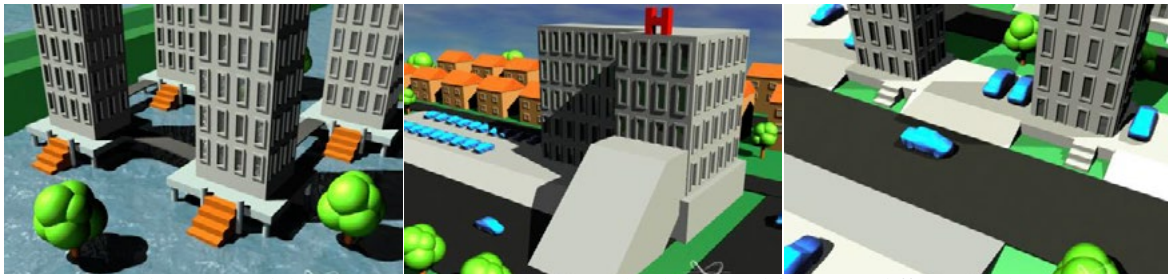
Figure 4: Building elevated: building elevated on poles, a non-livable ground floor, or a difference in level between street level and ground floor.
