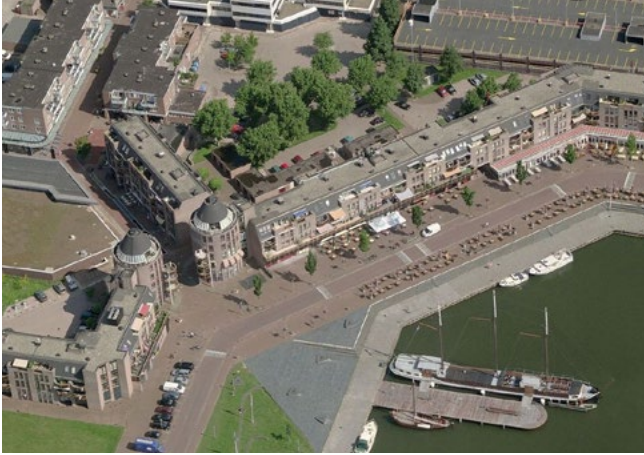
Figure 8.5.27: Early example of an unbreachable multi-functional dike (super dike) at Almere-Haven
