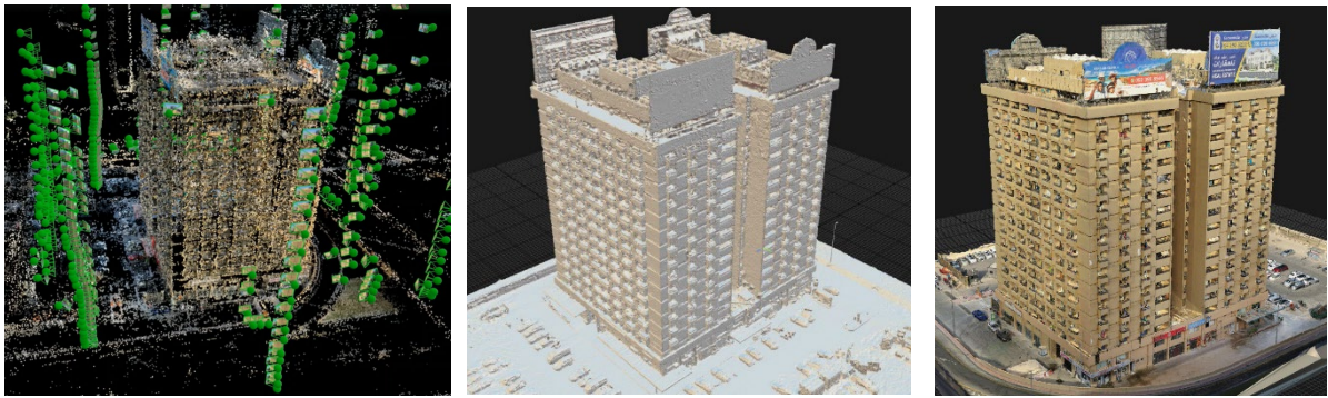
Figure 9. Data processing using photogrammetry RealityCapture software, © author(s).
