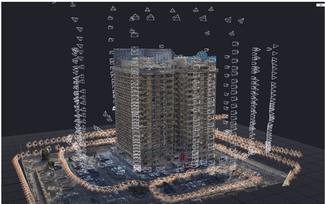
Figure 10. Point cloud of the 3D model consist of DJI drone images captured along vertical chains from above. The ground-level images highlighted in orange focus on the building's base, © author(s).
