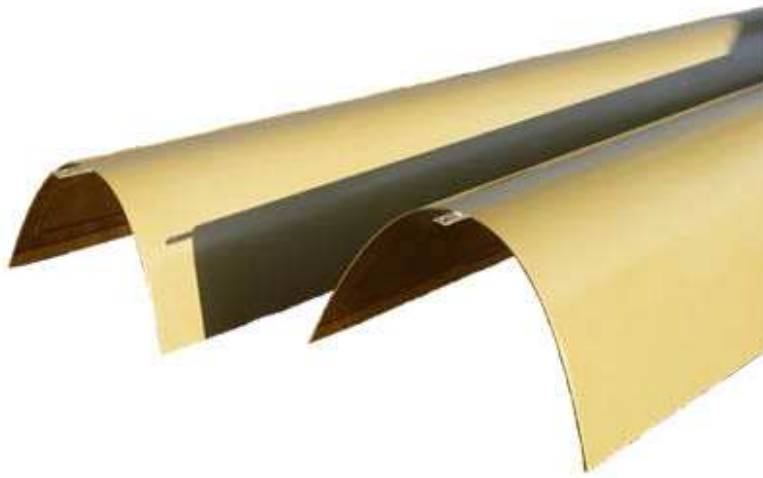
Figure 2.7: Glare leading edges as used in the Airbus A380 horizontal and vertical tail plane. Courtesy Fibre Metal Laminates centre of Competence.
