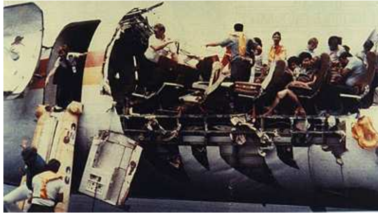
Figure 2.3: Accident with a Boeing 737 of Aloha Airlines in 1988 due to multiple site damage showing the importance of fatigue for ageing aircraft and of proper inspection and maintenance.
