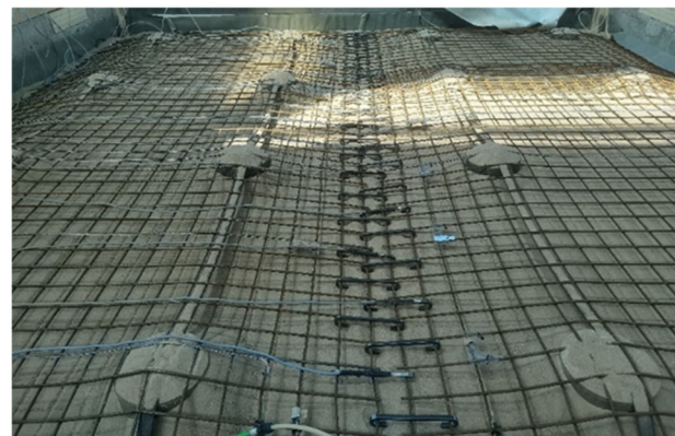
Figure 2. The large-scale test set-up showing the deformed steel mesh during excavation after test performance. Some of the 16 piles with a diameter of 225 mm and instrumentation are visible (2023, TU Darmstadt Geotechnical Test Pit facility)
