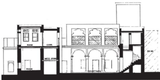
Figure 12, section through courtyard barajeel house (Damluji, 2006, p.187).
