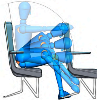
Figure 26: Reaching for something under seat in front in 32° seat pitch aircraft seat - side view
