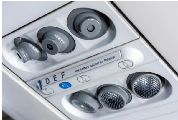
Figure 121: PSU lights, seats & ventilation (Knuth, 2023)
