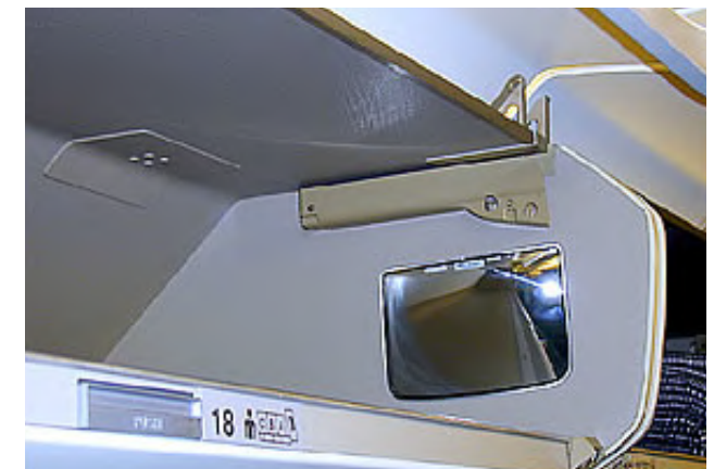
Figure 45: Mirror in overhead bins to help cabin crew check for lost luggage (Map, n.d.)
