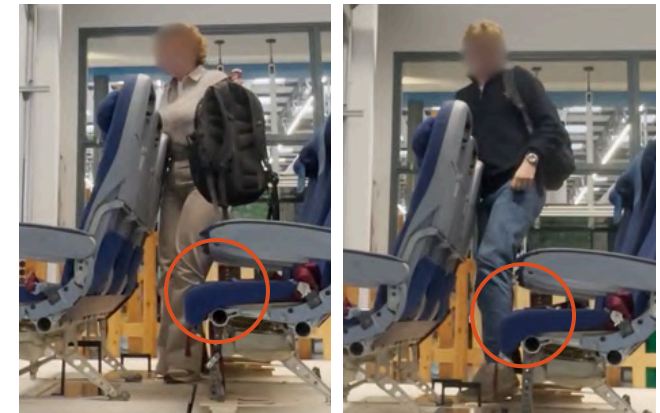
Figure 107: Test participants enter and exit the row of seats with their lower legs moving along the seat cushion.
