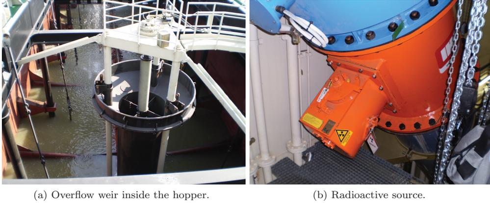
Figure 2.11: Overflow weir (left) and the radioactive source in the discharged pipe (right).
