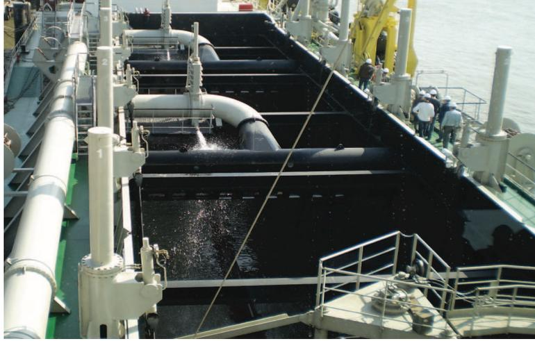
Figure 2.6: Example of a hopper.
